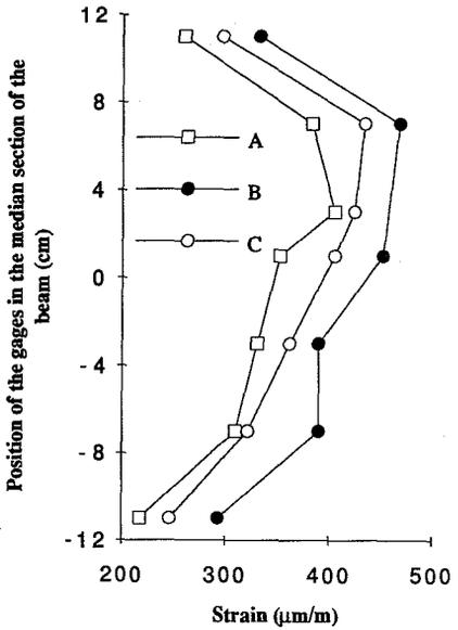
Figure 2 Strain values measured on the reinforced concrete beams after 1 year
