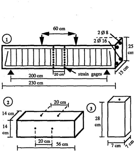
Figure 1 Description of the different types of concrete beams, prisms and bars
