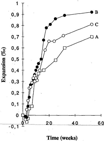
Figure 3 Measured expansions on the concrete bars (7 x 7 x 28)
