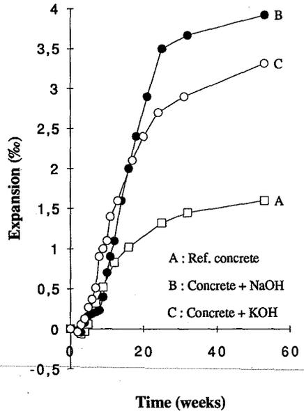
Figure 4 Measured expansions on the concrete prisms (14 x 14 x 56)
