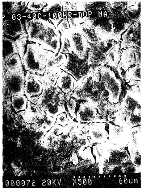
Figure 8 SEM micrograph of a massive gel (concrete + NaOH: 12 months)
