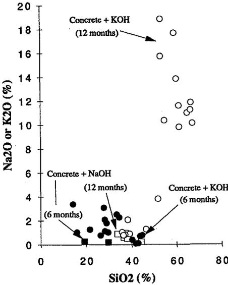
Figure 9  $\text{SiO}_2$  vs  $\text{Na}_2\text{O}$  or  $\text{K}_2\text{O}$  in the AAR gels (conc. + NaOH or + KOH after 6 & 12 months)
