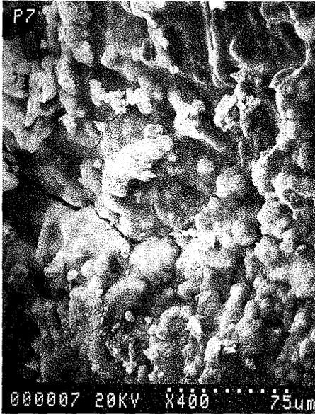
Figure 5 SEM micrograph of a massive gel (concrete + NaOH: 6 months)
