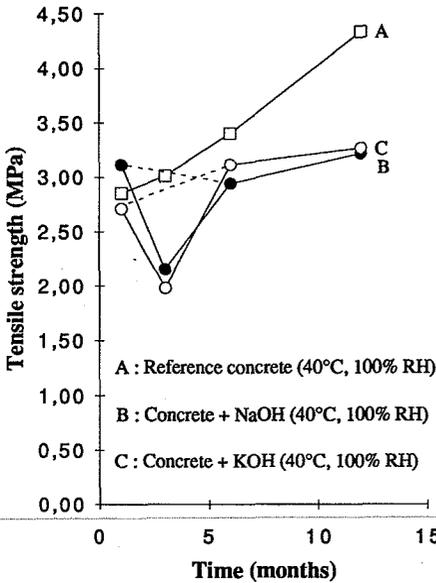
Figure 11 Variation of the concrete tensile strength with time
