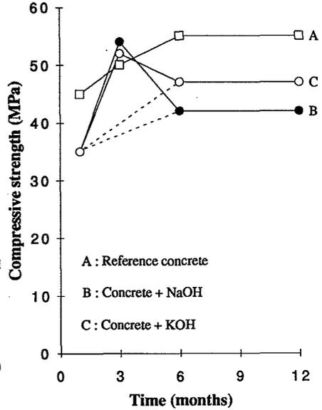
Figure 10 Variation of the concrete compressive strength with time
