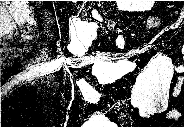
Figure 2 Petrographic microscope picture of core S-W 1 (area shown=1.5x2 mm 2 ); reaction of a porous chert grain with associated cracking and expulsion of gel
