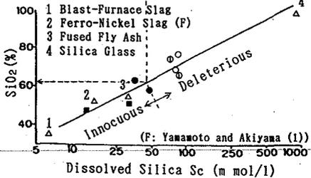
Figure 5 Chemical test of artificial and natural glasses (after Katayama et al. (16))
