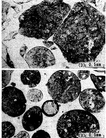
Figure 3 Spinifex texture of slag (D) and radial pyroxene texture of slag (B)
