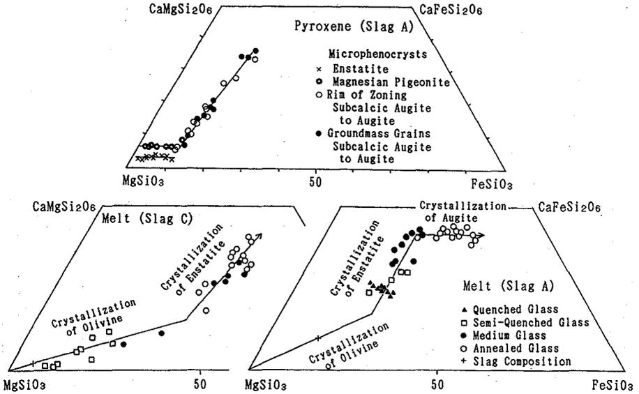
Figure 1 Compositional changes of pyroxene and melt in sintered, high-calcium, ferro-nickel slag (A), compared with molten low-calcium slag (C)
