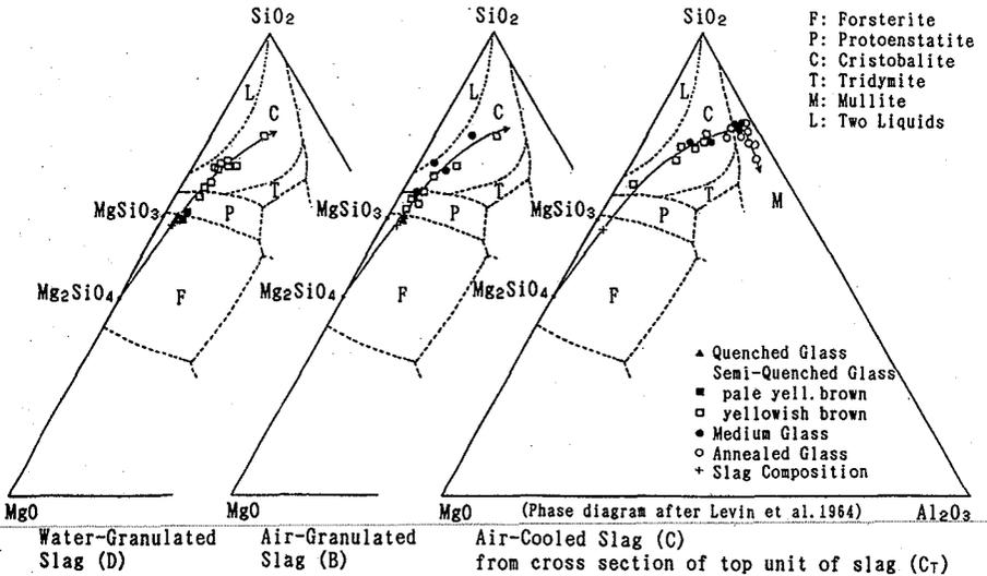
Figure 2 Compositional changes during cooling of melt in molten, low-calcium, ferro-nickel slags (B, C, D)
