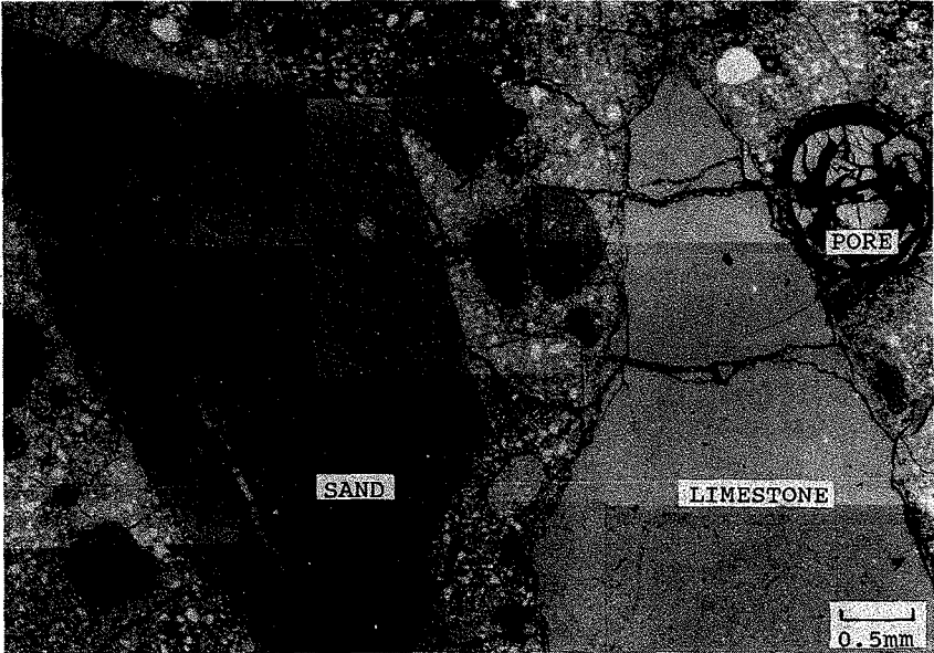
Figure 1 B.s.e. image of 7-year old concrete affected by A.S.R.
