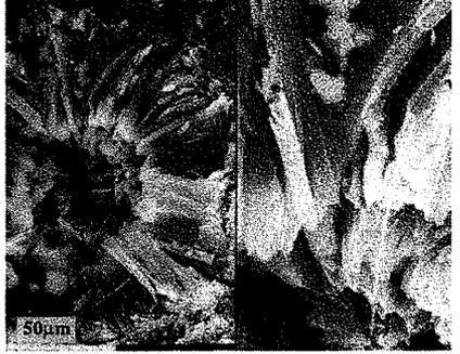
oriented ettringite normal to a bubble surface
