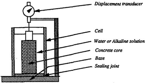
Figure 2 : Free expansion device
