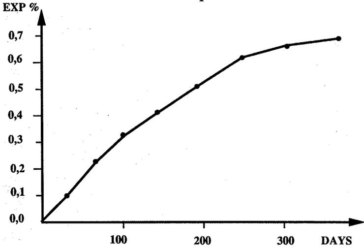
Figure 5 : Longitudinal expansion of the specimen subjected to free swelling.
