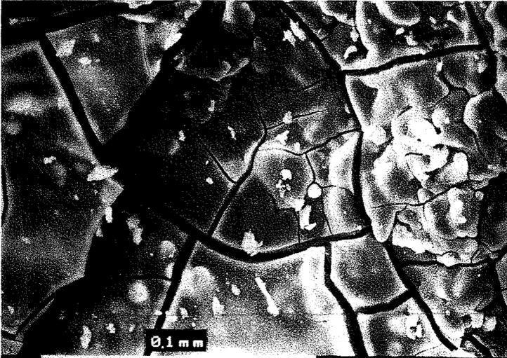
Photo 4 : Typical product of alkali-silica reaction.
