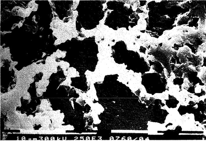
Photo 1 : Amorphous silica in dolomitic limestone.
