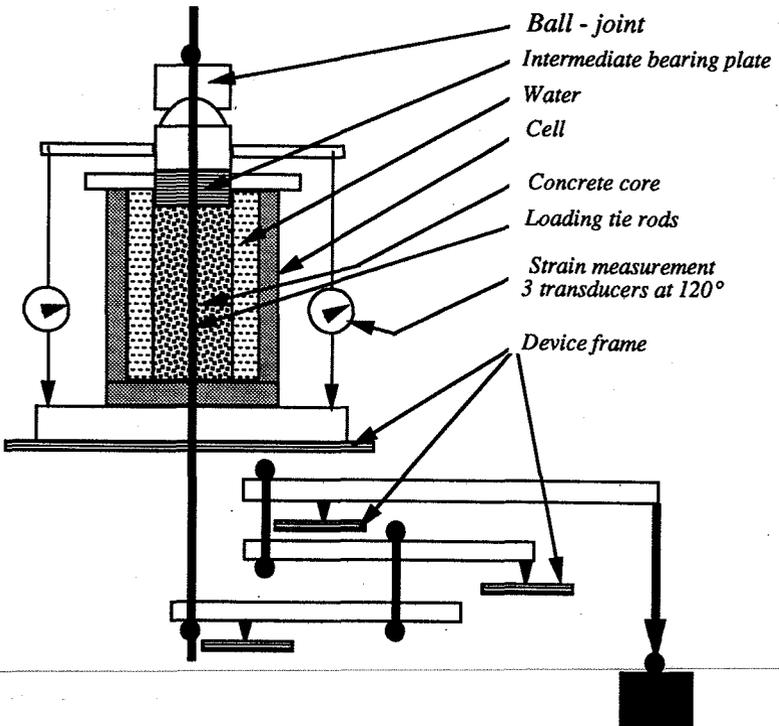
Figure 4 : Controlled stress expansion device
