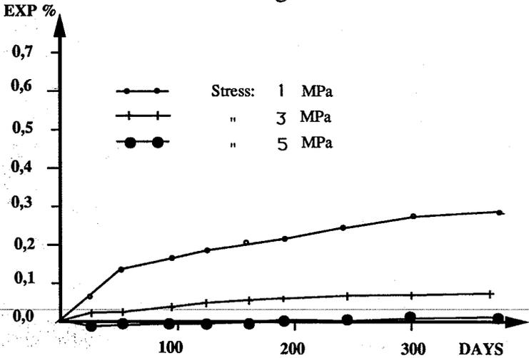
Figure 6 : Longitudinal expansions of specimen subjected to uniaxial stresses
