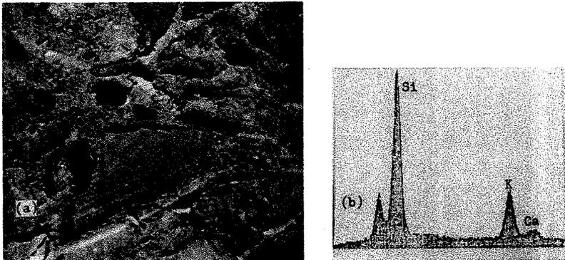
Fig. 3 (a) reacted aggregate, (b) composition of alkali-silica gel in reacted rim determined by EDXA
