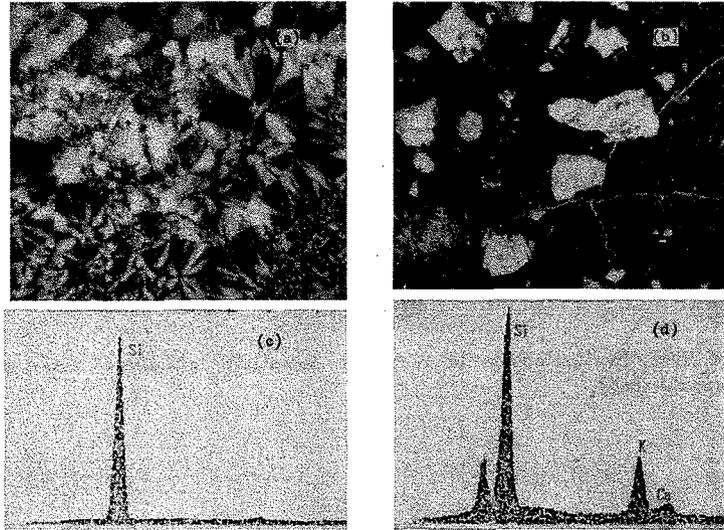
Fig.4 (a) chalcedony, (b)cracks, (c)Si-center of particle (by EDAX), (d)Si, K-reacted rim (by EDAX).
