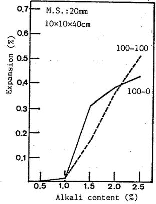
Fig. 4 Relationship between expansion and alkali content
