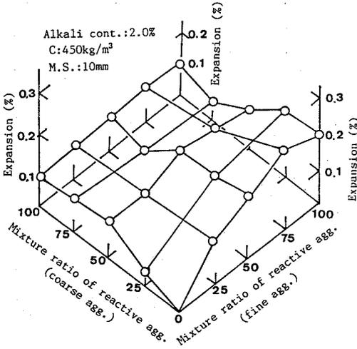
Fig. 3 Relationships between expansion and mixture of reactive aggregate
