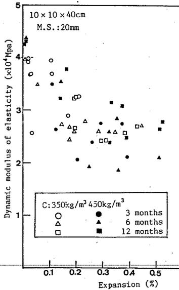
Fig. 5 Relationship between dynamic modulus of elasticity and expansion
