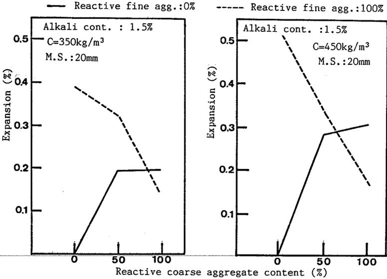
Fig.2 Relationship between the expansion of concrete and the ratio of reactive to
