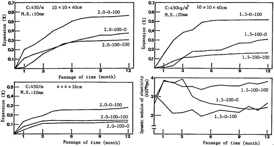
Fig.1 Change of expansion and dynamic modulus of elasticity with passage of time
