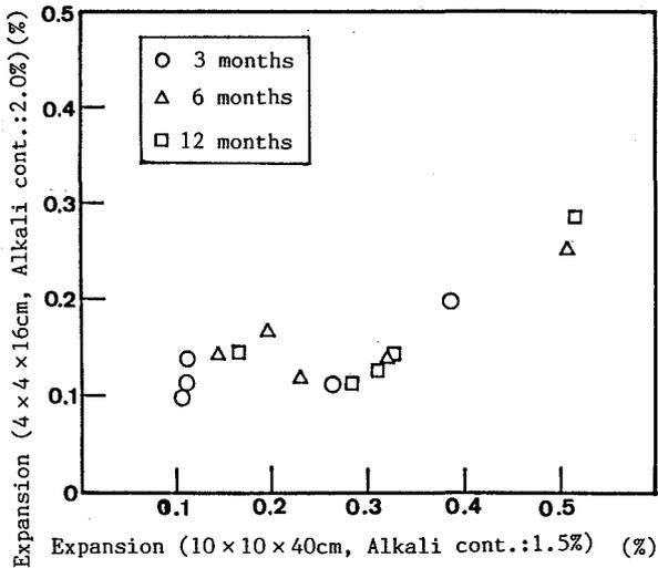
Fig. 8 Relationship between expansion of normal specimens and 4x4x16cm specimens
