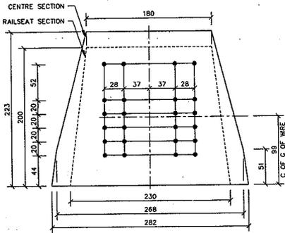
Figure 1 Reinforcing wire layout of Saldanha sleepers, 24 x 4 mm wires
