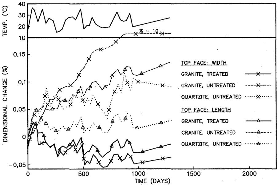
Figure 5 Dimensional changes measured on the top faces of untreated halves of sleepers and one half that was treated with a water repellent
