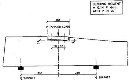
Figure 2 Support for rail seat repeated load test
