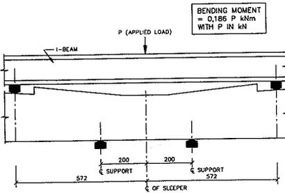
Figure 3 Support for sleeper centre repeated load test
