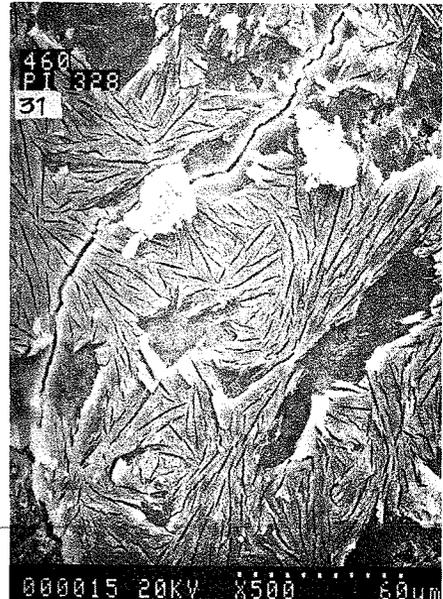
Figure 4 SEM micrograph of massive ettringite + thaumasite + calcite patch on a reactive aggregate
