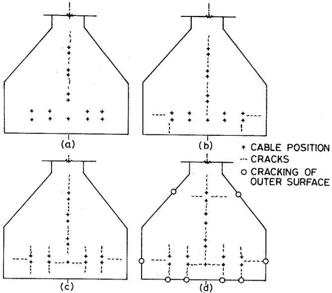
Figure 3 Crack Initiation, predicted by Finite Element Analysis
