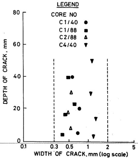
Figure 5 Relationship between crack width and crack depth
