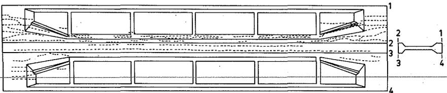
Figure 2 Cracking of PSC beams shown on developed surface
