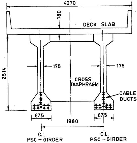
Figure 1 Cross-section of bridge girder, dimensions in mm
