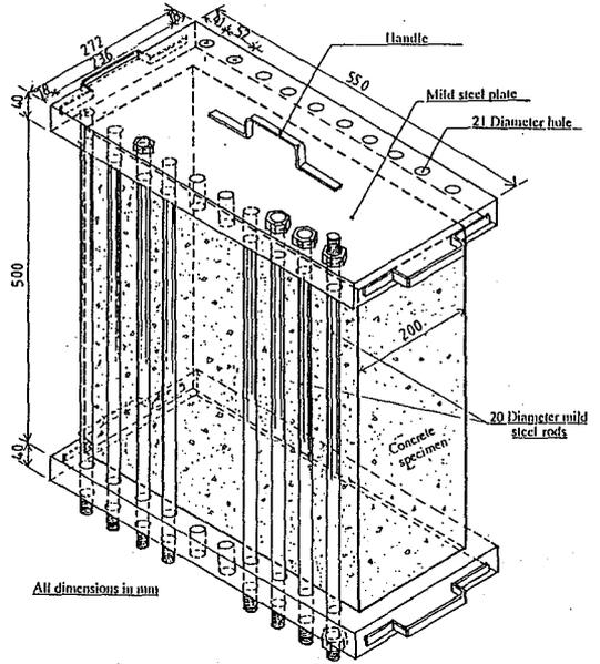
Figure 2 Preloading system
