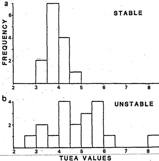
Figure 4a,b. Histograms showing the distribution of the true extinction angles when related to the textural stability of the quartz grains. a) stable textures, b) unstable textures.
