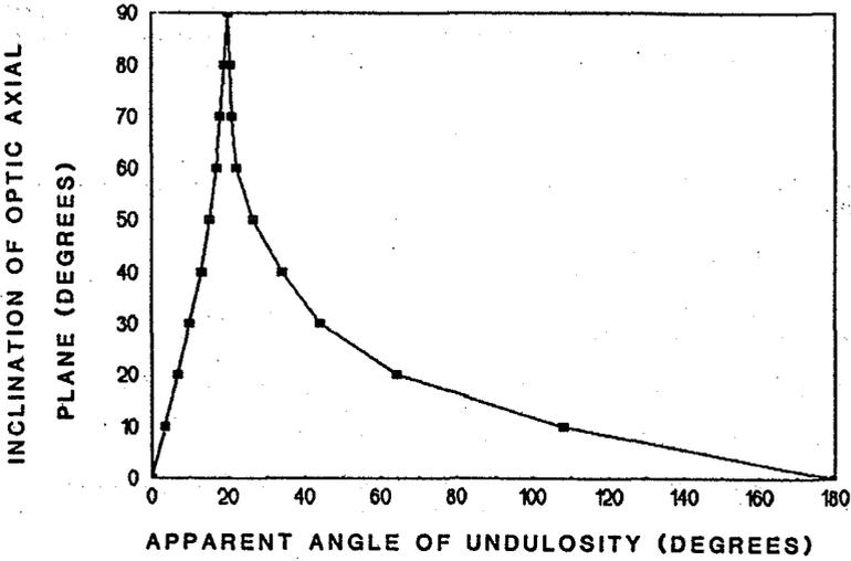
Figure 1. Graphical representation of the possible apparent extinction angles for a true extinction angle of 20°. Possible values plot on or below the curve.
