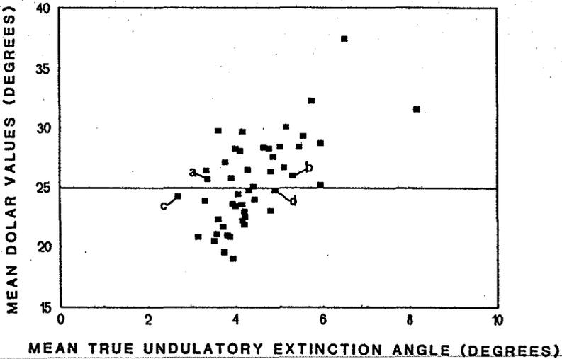
Figure 2. Graphical representation of the comparison between the values for the method prescribed in the guide-lines and the corresponding true angle of extinction.
