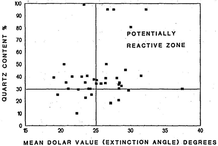
Figure 3. Graph showing the Concrete Society guide-line values for potentially reactive quartz and the distribution found in the examined samples.
