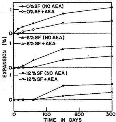
Figure 3 Effect of AEA on ASR expansion of mortar bars
