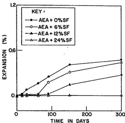
Figure 2 Effect of SF on ASR expansion of mortar bars in the presence of AEA
