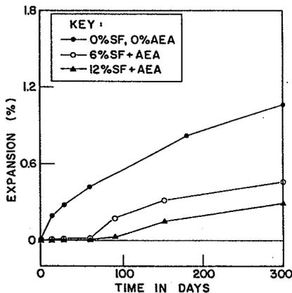
Figure 4 Effect of combined AEA and SF on ASR expansion of mortar bars
