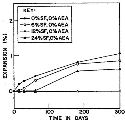
Figure 1 Effect of SF on ASR expansion of mortar bars in the absence of AEA
