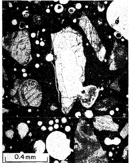
Figure 6 Optical micrograph of opal in mortar bars with 6% SF but no AEA
