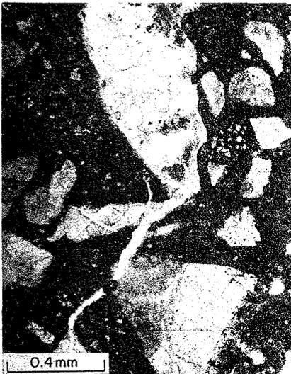
Figure 7 Optical micrograph of opal in mortar bars with AEA but no SF
