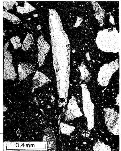
Figure 8 Optical micrograph of opal in mortar bars with AEA and 6% SF
