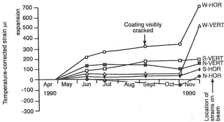
Fig. 3: Measured expansion of the surface of a 25 year old R.C. portal beam
