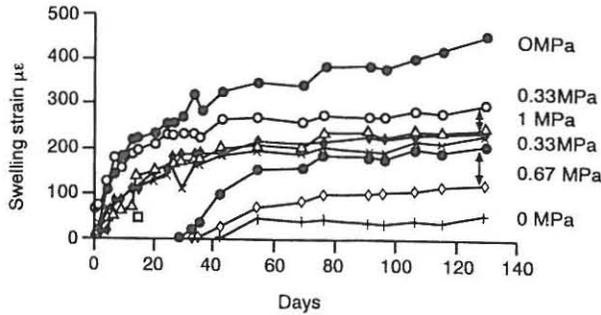
Fig. 5: Swell-under-load versus time relationships for pre-demolition cores of 25 year old concrete
