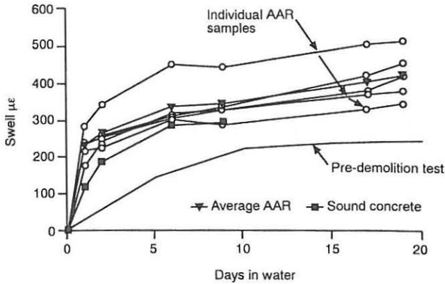
Fig. 8: Free swell of cores in 1998 tests compared with pre-demolition test (Fig.4)
