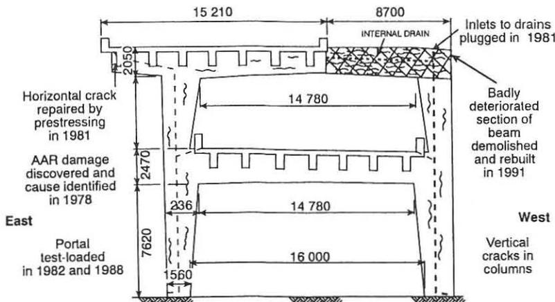
Fig. 1: Main dimensions (mm) of the two-level portal frame showing various repair procedures and tests (1981 to 1991) (elevation looking south)
