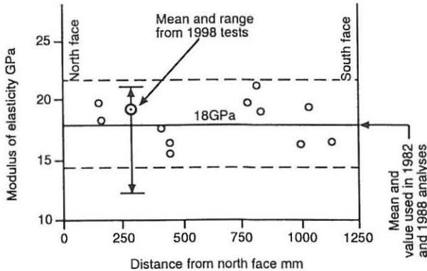
Fig. 6: Modulus of elasticity measurements on pre-demolition cores from portal beam
