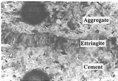
Fig. 11: Ettringite deposited at the aggregate/cement paste interface (1 division = 2 $\mu$ m)
