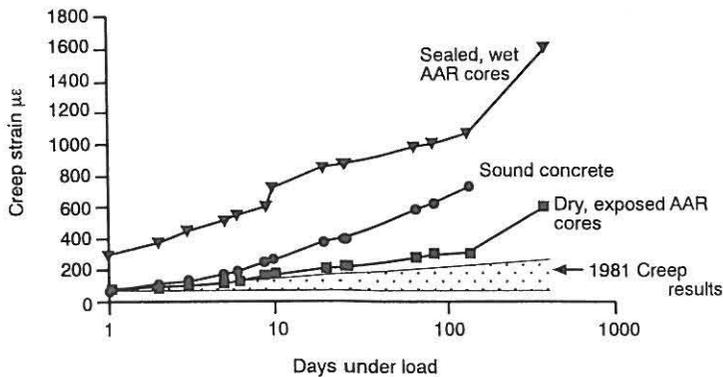
Fig. 9: Comparison of 1998 and 1981 (Figure 7) creep results
