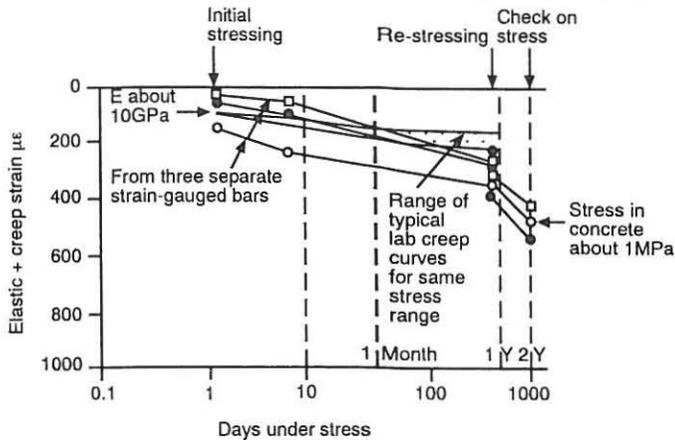
Fig. 7: Field creep curves measured on cantilever nib repaired by prestressing
