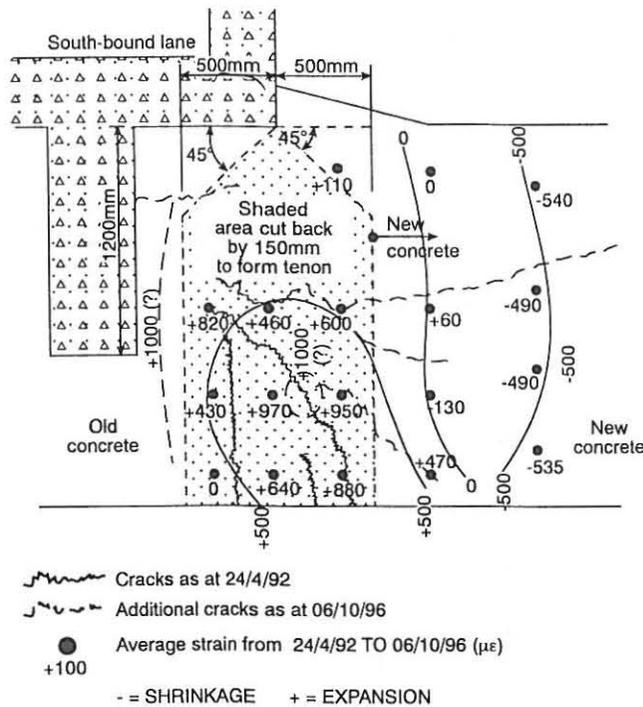
Fig. 4: Average strains and cracking recorded 5½ years after repairing the portal beam
