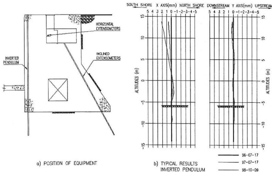
Fig. 2: Monitoring equipment for a typical monolith
