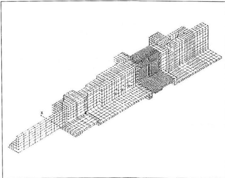
Fig.3: Finite element Model 3, phase 2: Monolith 7N
