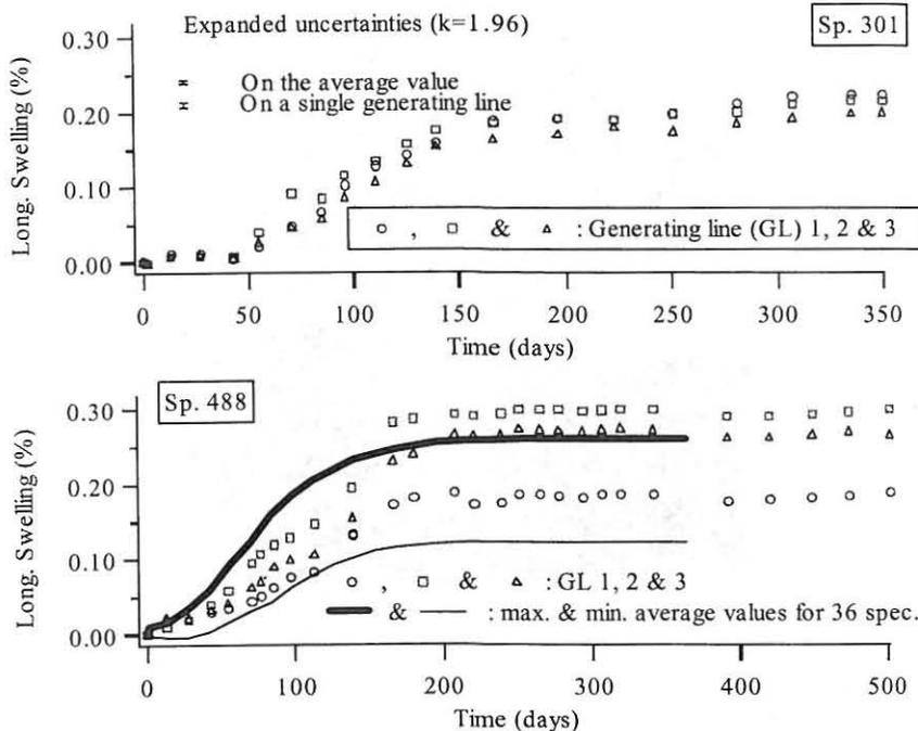
Fig. 2: Heterogeneity of reactive concrete cylinders longitudinal swelling. The continuous curves represent the maximum and minimum average longitudinal swelling (averaged on three measurements) for thirty-six cylinders kept in similar storage conditions (38°C, 95 to 100% RH).
