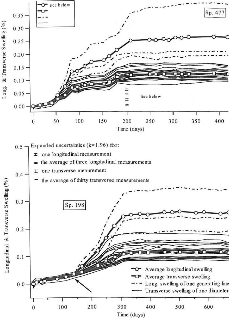
Fig. 4: Longitudinal versus transverse swelling for sp. 477 at 38°C and sp. 198 at 23°C
