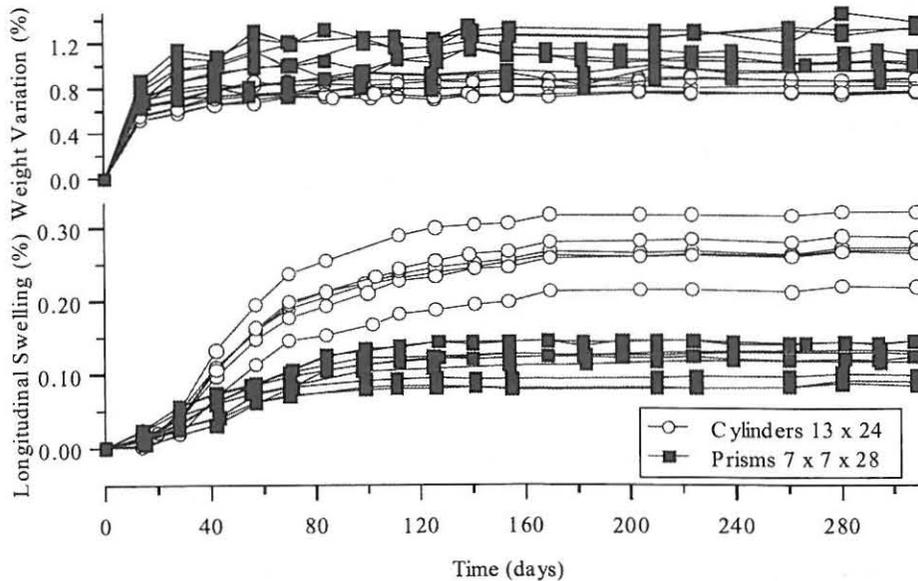
Fig. 7: Comparison between the longitudinal swelling of cylinders and prisms
