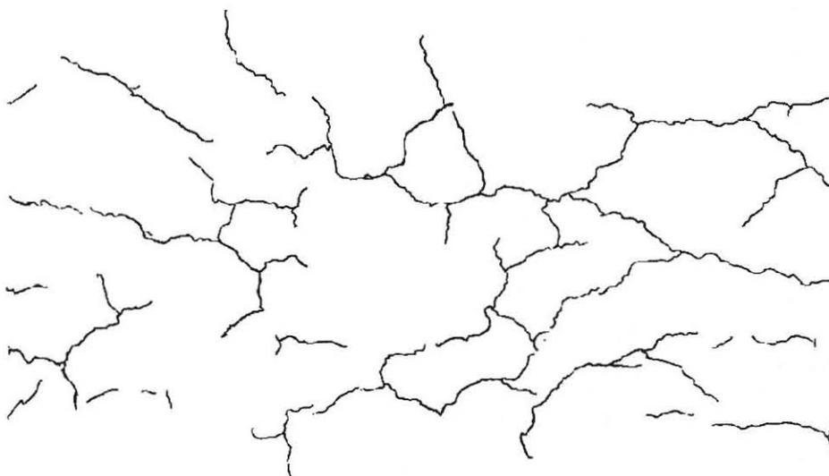
Fig. 6: Example of map cracking on a cylinder (cracks width is not represented) - Horizontal cracks are more numerous than vertical ones.
