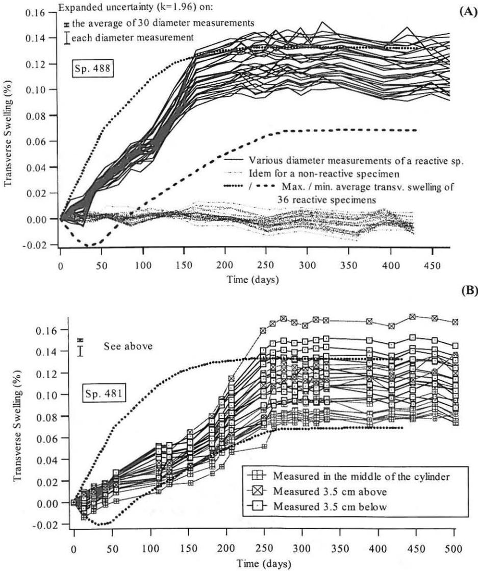
Fig. 3: Heterogeneity of reactive concrete cylinders (24 cm high, 13 cm in diameter) transverse swelling. The dash curves represent the maximum and minimum average transverse swelling (averaged on thirty measurements) for thirty-six cylinders kept in similar storage conditions (38°C, 95 to 100% RH).
