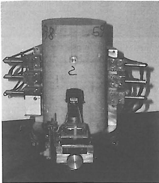
Fig. 1: LCPC diameter variations measurement device
