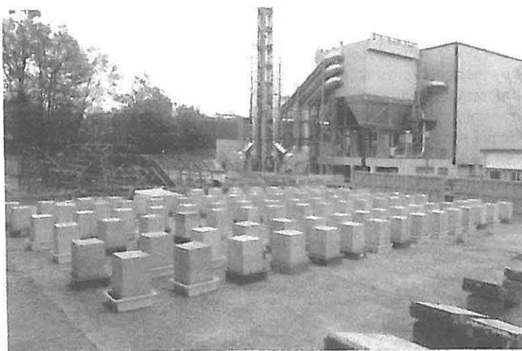
Fig. 1: BRE external exposure site for 500x300x300 mm concrete blocks.
