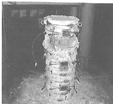
Fig. 4: RC column with the breaking down of PC wire at failure
