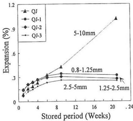
Fig. 3: The expansion curve of dolomitic limestone from Shandon
