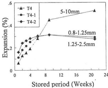
Fig. 5: The expansion curve of dolomitic limestone from Hebei
