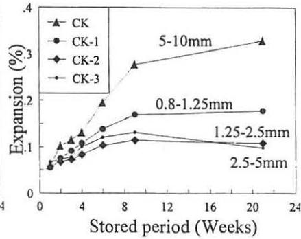
Fig. 6: The expansion curve of dolomitic limestone from Kingston
