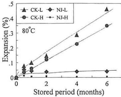
Fig. 9: Comparison test for low and high alkali cements at 80°C (40 by 40 by 160 mm).
