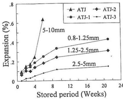
Fig. 1: The expansion curve of argillaceous dolomite from Tianjin
