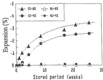
Fig. 8: A comparison test for typical reactive and inert rocks at 80°C and 40°C.
