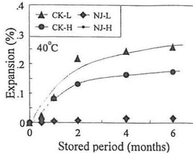
Fig. 10: Comparison test for low and high alkali cements at 40°C (40 by 40 by 160 mm).
