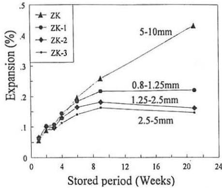
Fig. 4: The expansion curve of dolomitic limestone from Sichuan
