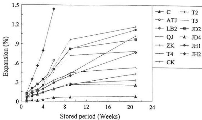
Fig. 7: The expansion curves of various carbonate rocks in alkali solution at 80°C (1M NaOH, 40 by 40 by 160 mm)
