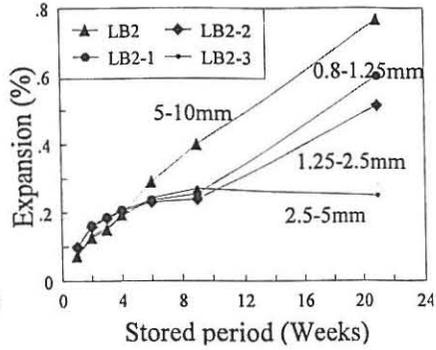
Fig. 2: The expansion curve of dolomitic limestone
