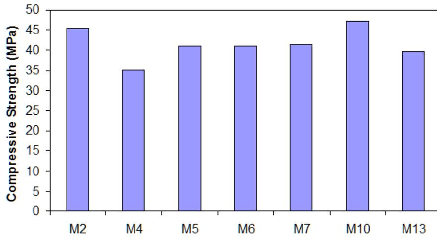
Figure 4: Residual compressive strength of mixtures ( $w/c = 0.33$ ).
