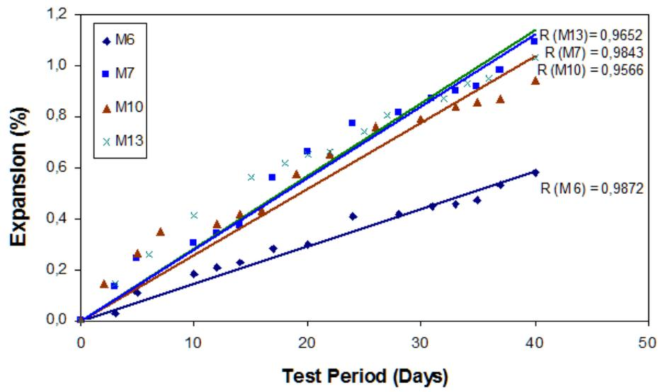
Figure 3: Expansion-time graph of samples containing fine and coarse aggregate.
