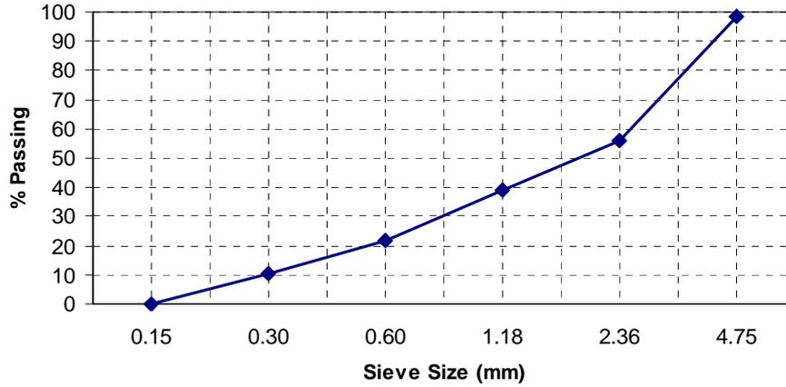
Figure 1: Grading of fines.
