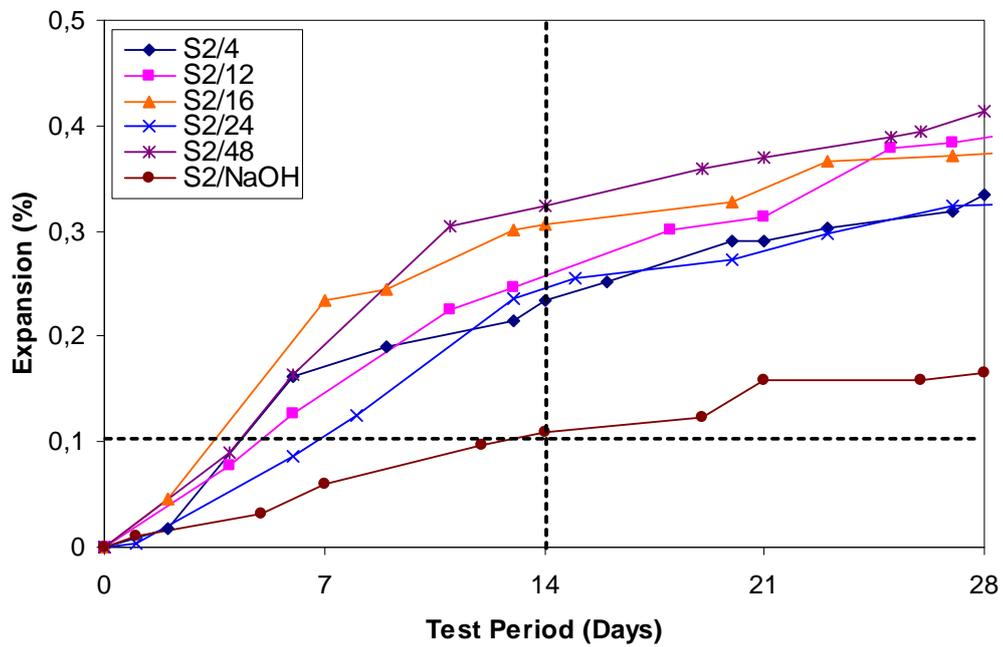
Figure 2: Expansion-time graph of S2 specimens having different pre-curing periods (AMBT method).
