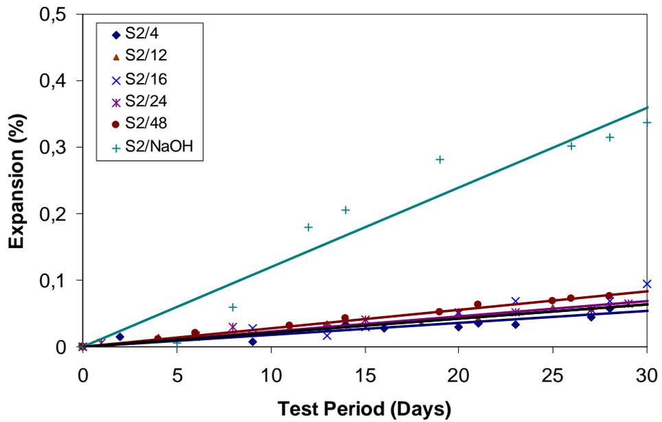
Figure 4: Expansion-time graph of S2 specimens having different pre-curing periods (CMT method).
