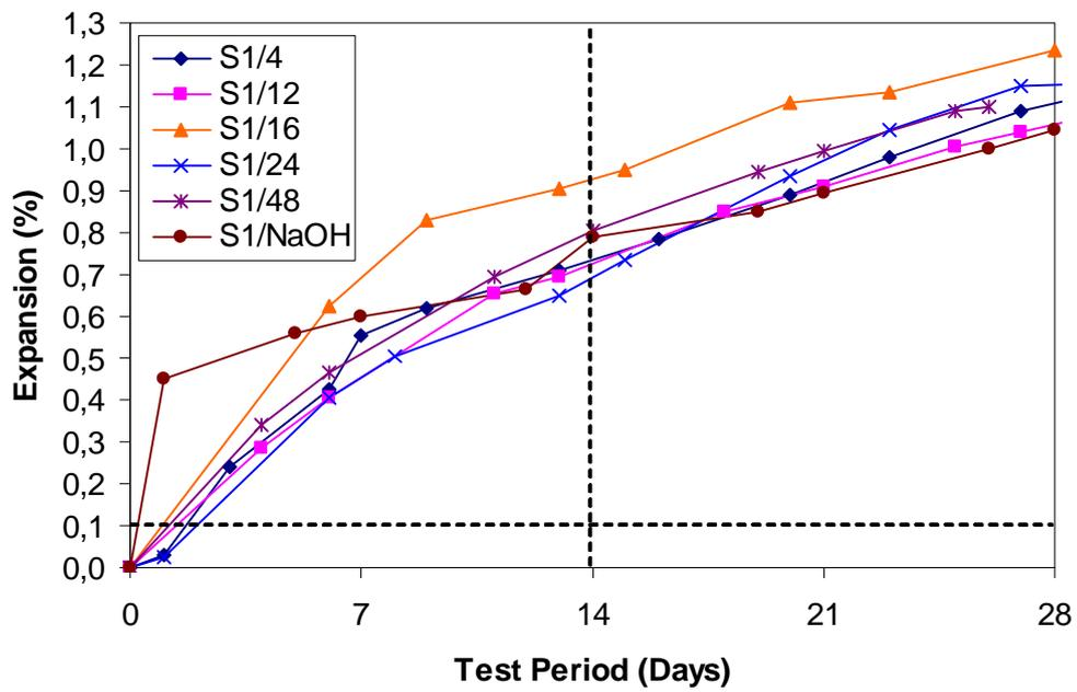
Figure 1: Expansion-time graph of S1 specimens having different pre-curing periods (AMBT method).
