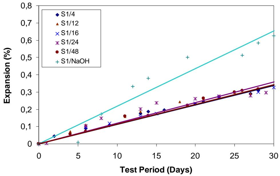
Figure 3: Expansion-time graph of S1 specimens having different pre-curing periods (CMT method).
