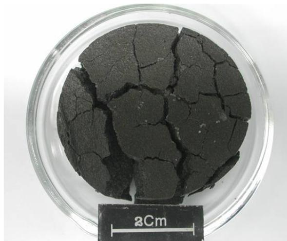
Figure 2: Photograph of a 20%wt DSF blended cementitious paste sample after a few days immersion in water during the leaching experiment.
