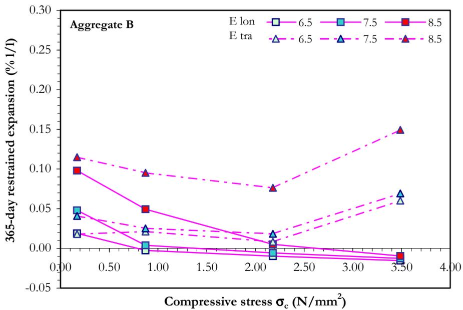
Figure 6: Ultimate restrained longitudinal expansion vs. compressive stress (aggregate B)
