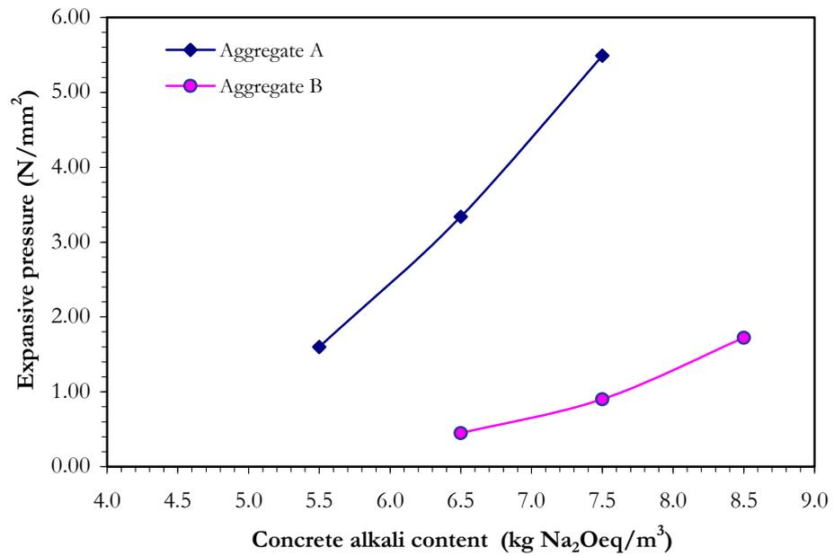
Figure 8: Expansive pressure vs. concrete alkali content after one year of measurements
