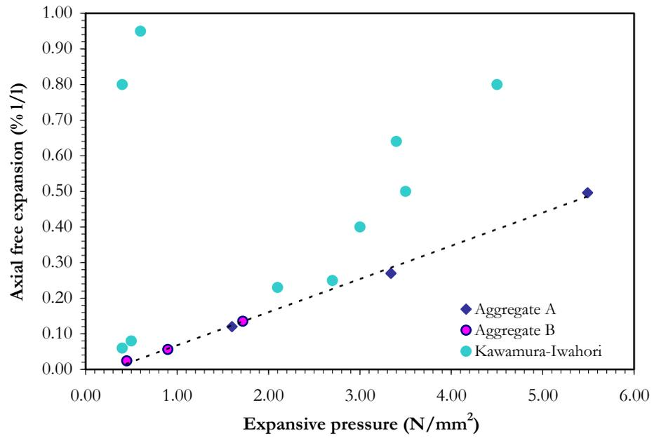
Figure 7: Axial free expansion vs. expansive pressure after one year of measurements (experimental data compared with previously published data from literature)
