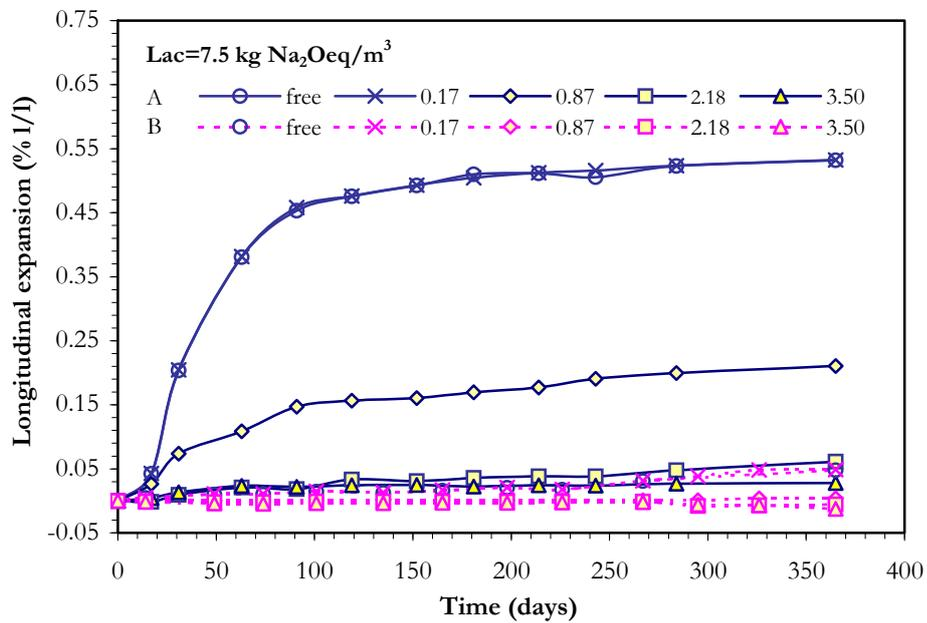
Figure 2: Length change vs. time for concrete prisms (alkali content = 7.5 kg Na<sub>2</sub>Oeq/m<sup>3</sup>) under different test conditions (free and restrained expansion)
