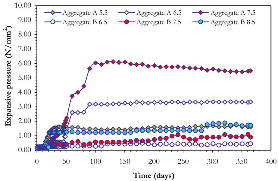
Figure 3: Development of “free” expansive pressure (under the lowest restraining stress of 0.17 N/mm<sup>2</sup>) for all concrete mixes investigated
