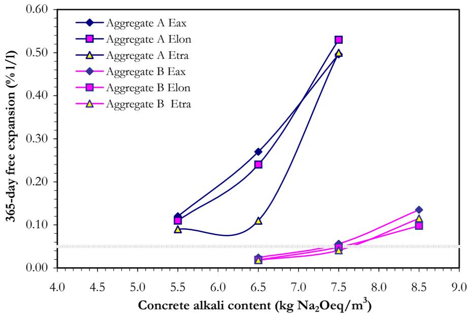
Figure 4: Ultimate free expansion (axial, longitudinal, transversal) vs. concrete alkali content
