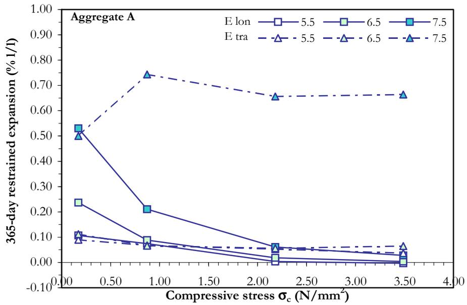
Figure 5: Ultimate restrained longitudinal expansion vs. compressive stress (aggregate A)
