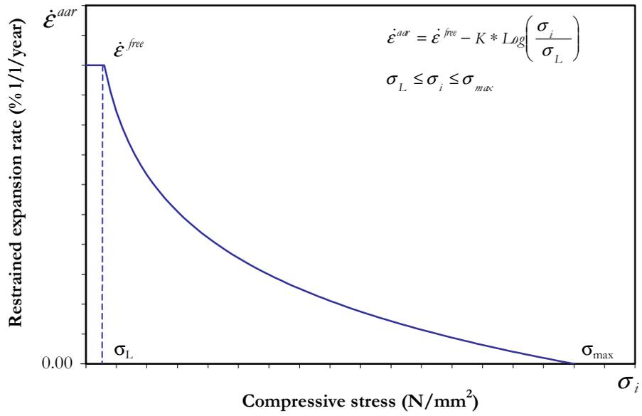
Figure 10: Relationship between concrete strain growth rate  $\dot{\epsilon}^{aar}$  and principal stress  $\sigma_i$  in ASR [10] [11]
