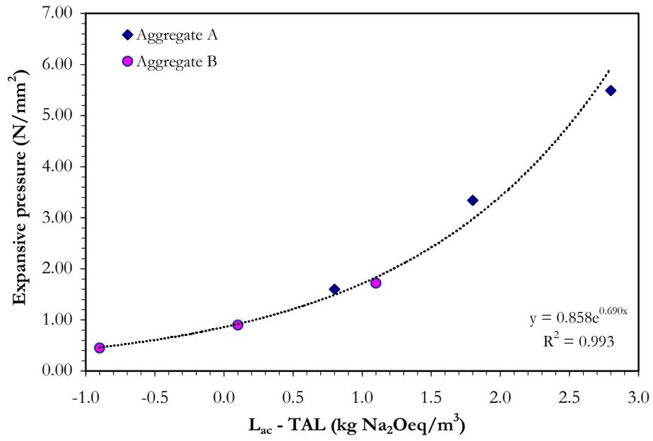
Figure 9: Expansive pressure vs. driving force for ASR development
