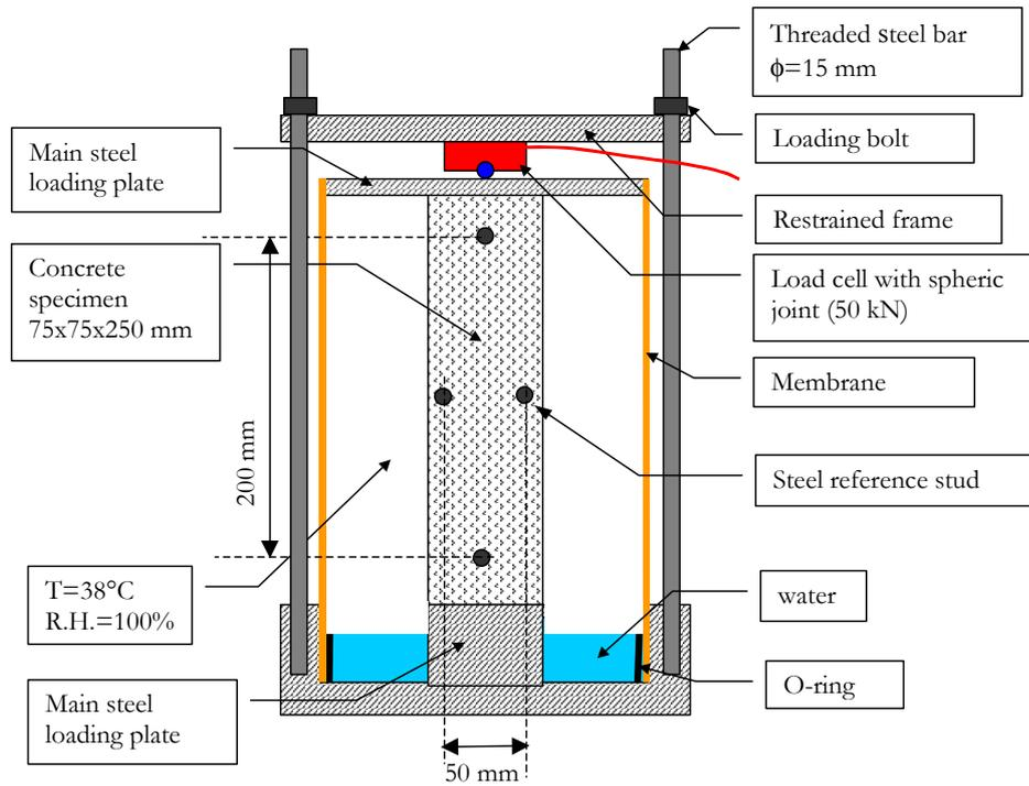
Figure 1: Schematic lay-out of the steel pressure cell for measuring expansion and expansive pressure
