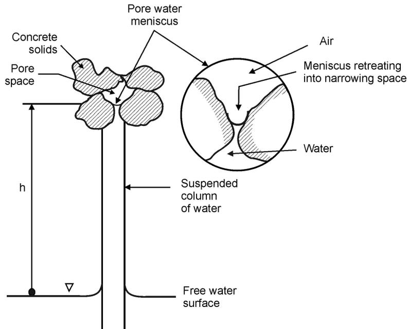
Figure 5: Capillary model of partly saturated concrete.
