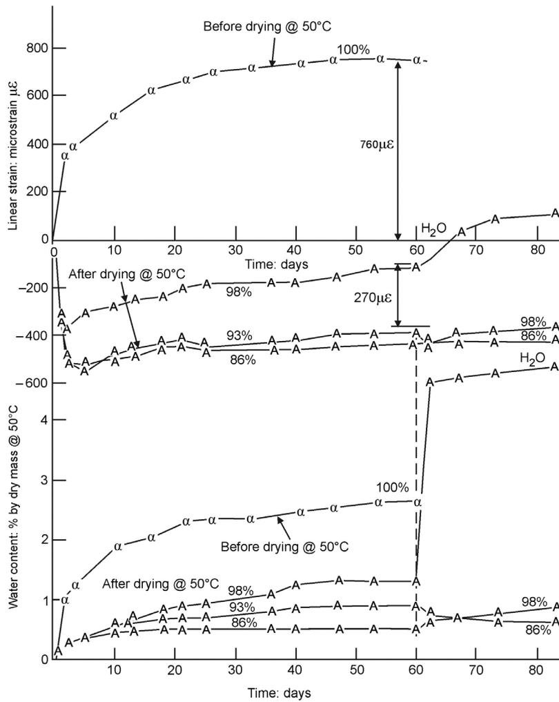
Figure 1: Behaviour of specimens "A" during exposure to relative humidities of 86% to 98% at 20°C after drying at 50°C. (" $\alpha$ " shows behaviour of specimen exposed to nominal 100% RH before drying at 50°C.) ("A") specimens were AAR-affected.
