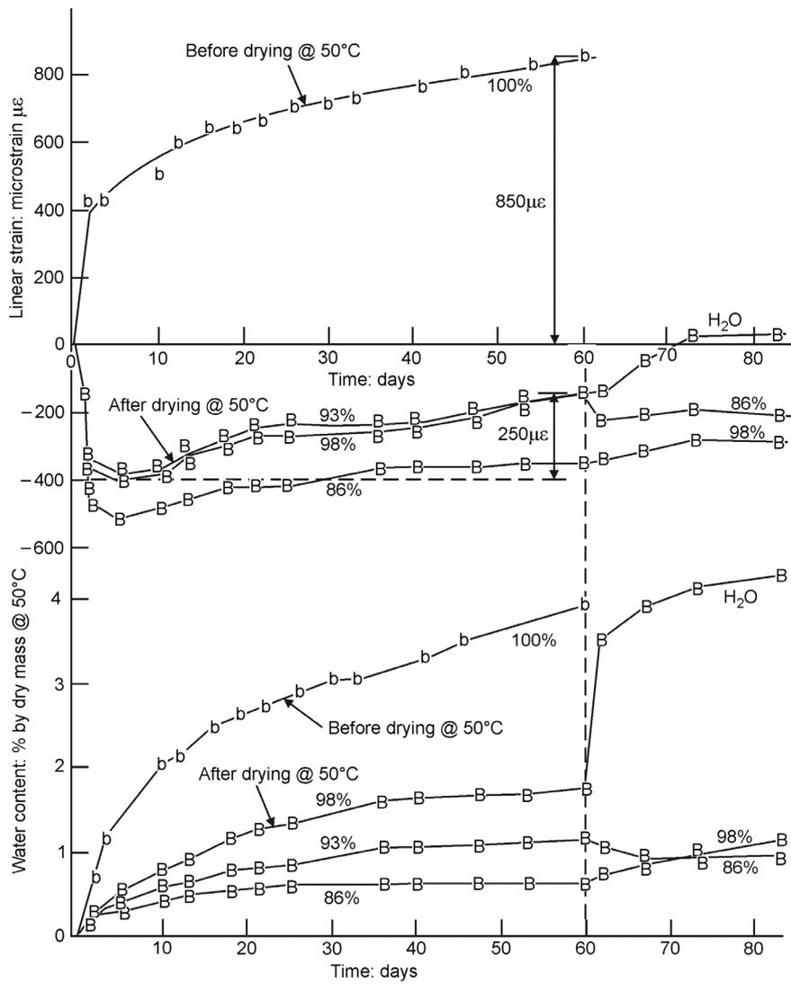
Figure 2: Similar to Figure 1, but for specimens "B" ("B" specimens were AAR-affected).
