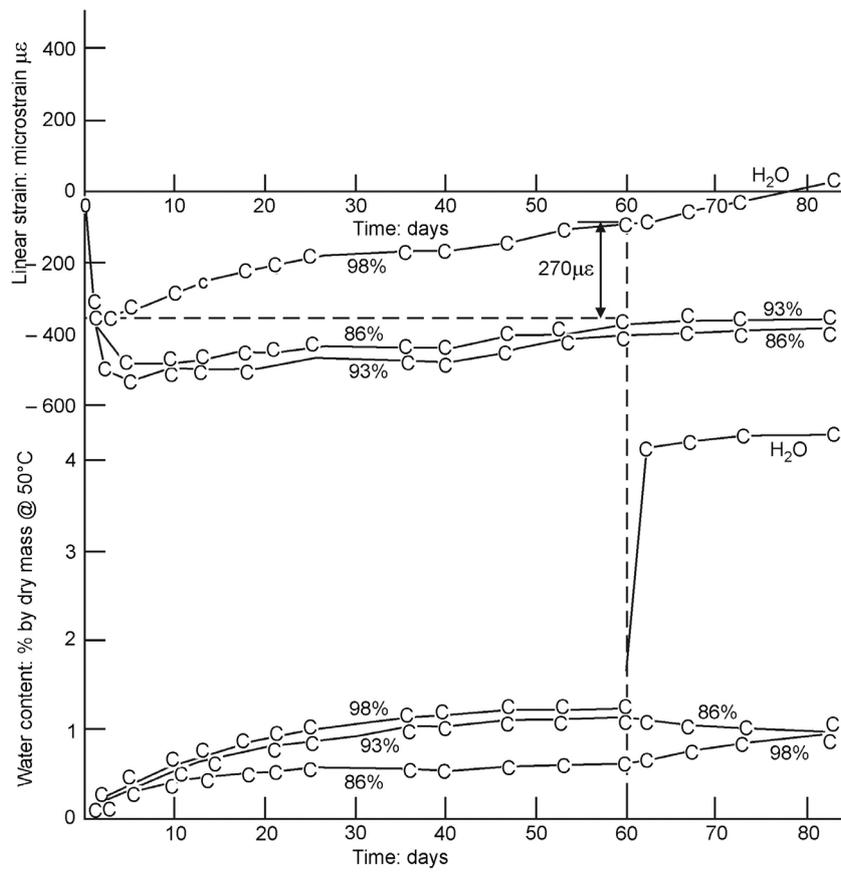
Figure 3: Similar to Figures 1 and 2, but for specimens "C" (Specimens "C" have dolomite aggregate and are not affected by AAR).
