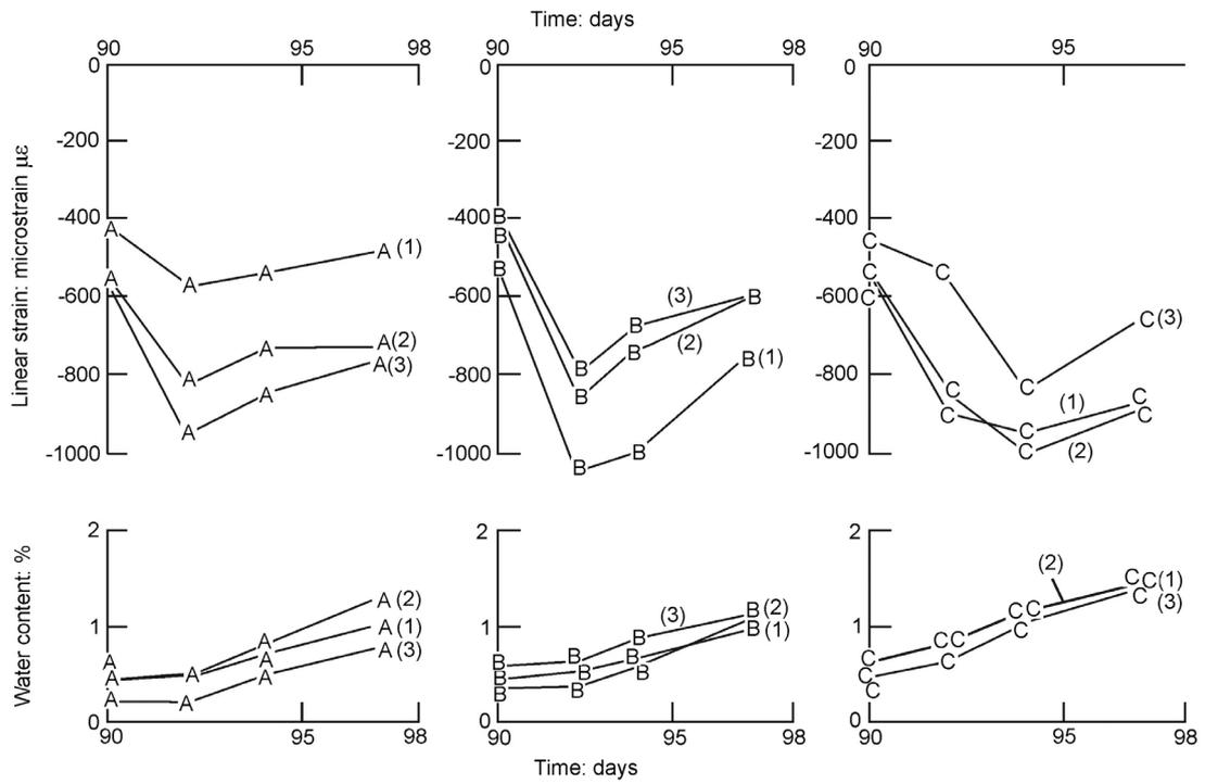
Figure 4: Behaviour of specimens after re-drying at 50°C followed by exposure to 93% relative humidity, at 20°C. In each case, zero strain and water content are the same as in Figures 1, 2 and 3. (The numbers (1), (2) and (3) allow water content and linear strain curves to be matched).
