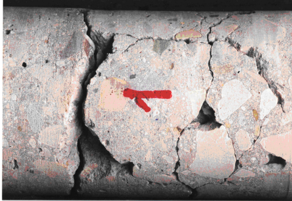
Figure 1: Core (diameter 100 mm) extracted from a structure affected by AAR: it appears heavily cracked.
