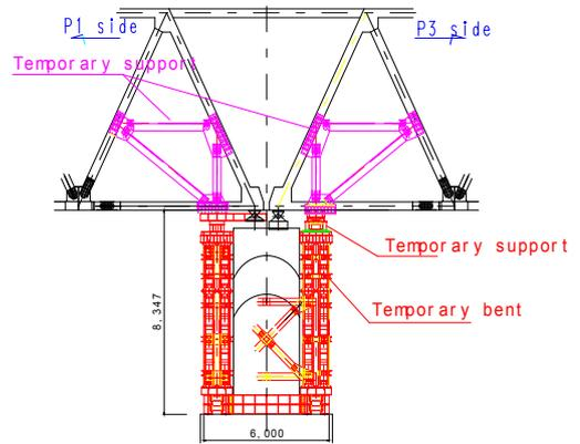
Figure 13: Design of temporary bent
