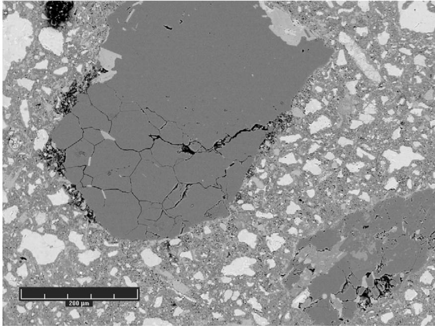
Figure 1: Micrograph of a sample after a MICROBAR test. One can clearly see the cracks initiating at the zones within the aggregates which reacted.
