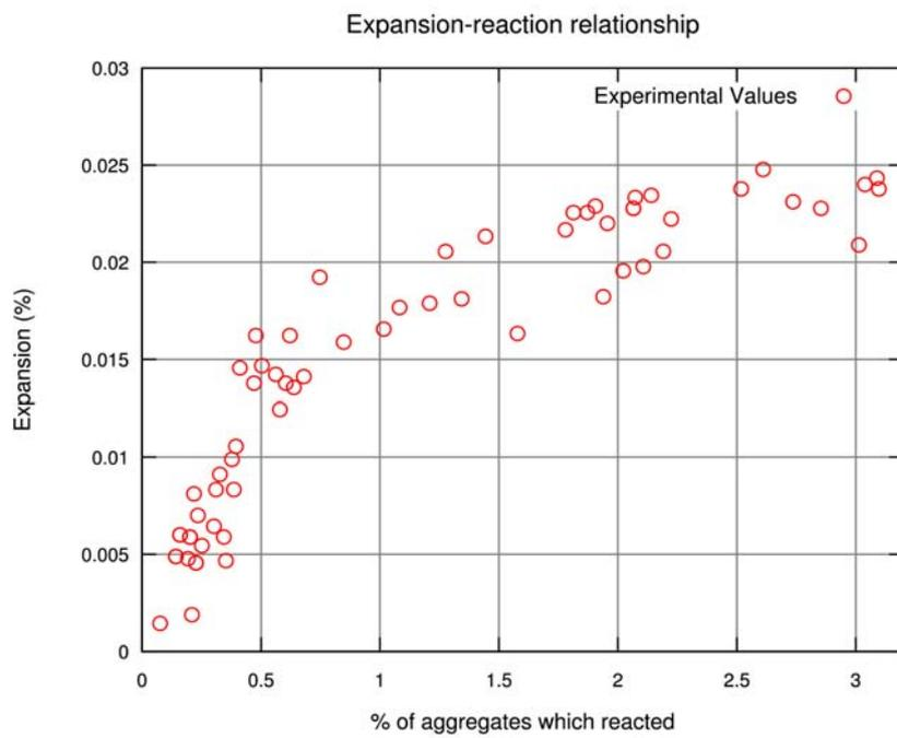
Figure 2: Experimental relationship between measured free expansion and measured reacted fraction. Both mortar and concrete expansions values are reported in this graph, after renormalisation of the concrete expansion values with respect to the relative aggregate content. Adapted from Ben Haha[8].
