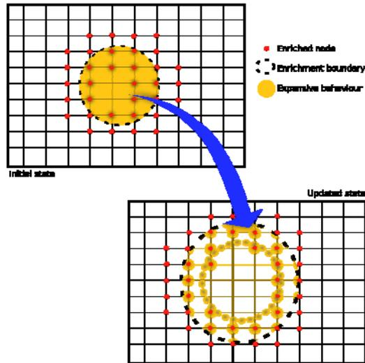
Figure 3: Update of the enrichment scheme. Enrichment nodes are updated according to the new geometry. Expansive behaviour is attributed to the elements and part-elements within the reacted zones. The enrichment strategy is independent of the mesh and mesh type: here a quadragular regular mesh is shown for clarity.
