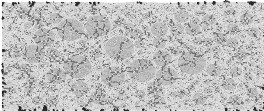
Figure 5: Map-cracks are highlighted in the simulation. In two dimensions, they are cracks initiating from the surface of the sample at regular intervals. This example is the result of a non-realistic simulation performed to highlight the mechanical consequences of the gel expansion.
