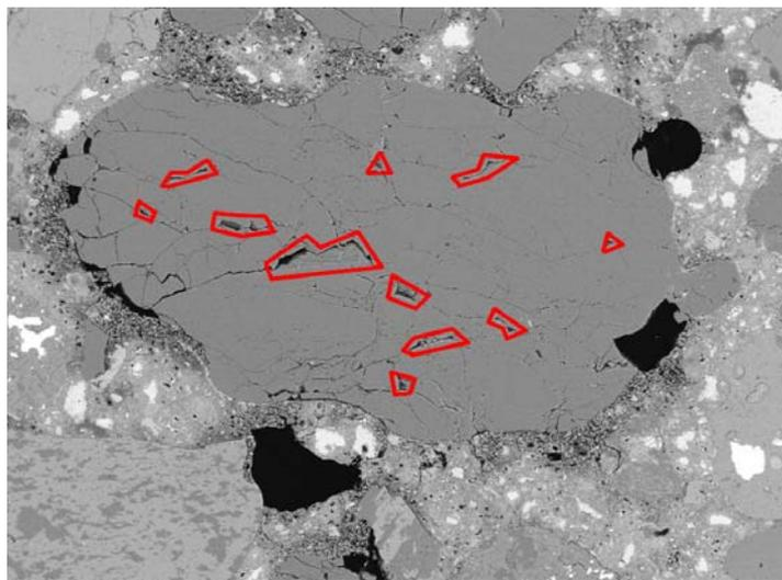
Figure 4: Star-like patterns originating from reactive zones are observed. Reactive zones are marked in red.
