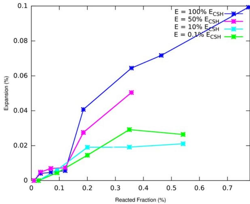
Figure 6: Simulated expansion-reaction curves. The parameter varied is the stiffness of the gel, all other parameters are kept constant. We see that simply varying this parameter does not affect the shape of the curve, but only scales it.
