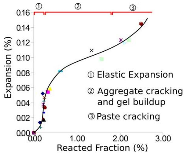
Figure 7: Experimental expansion-reaction curve (adapted from Ben Haha [8]). The phases in the ASR damage mechanism are highlighted.
