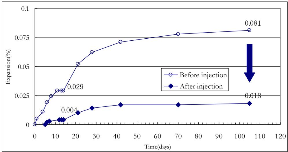
Figure 7: Results of the accelerated curing test at 40 degrees Celsius, RH 95%
