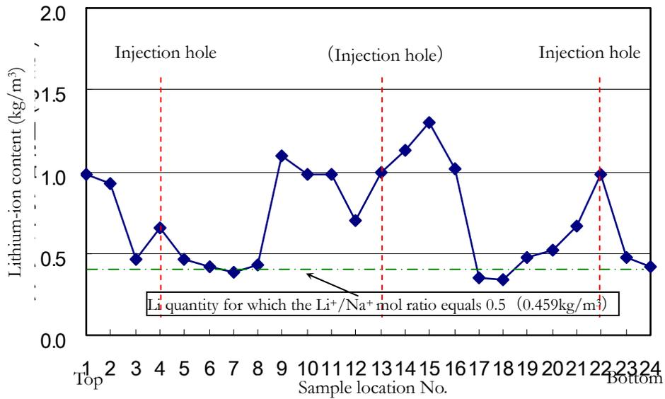
Figure 6: Lithium-ion is supplied over the amount required for ASR inhibition for a range of approximately 88% of the concrete interior.
