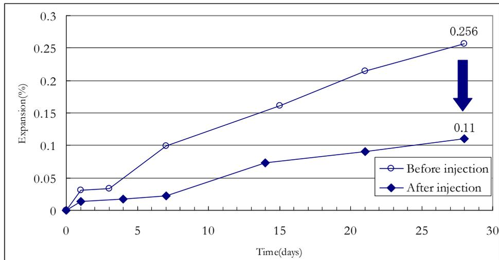
Figure 8: Results of the accelerated curing test at 80 degrees Celsius in a 1N NaOH solution
