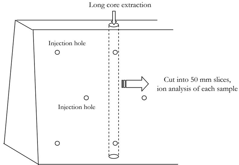
Figure 5: Extraction of lithium-ion analysis sample material
