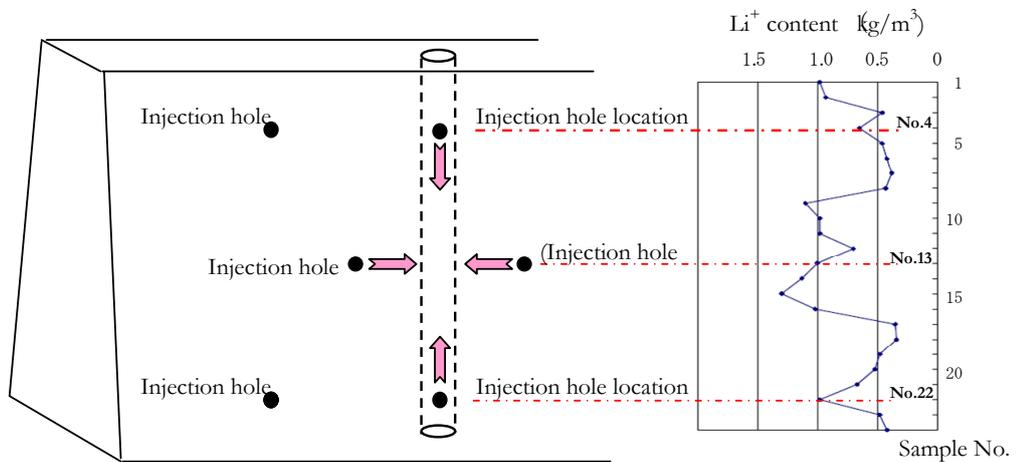
Figure 9: Relationship between extraction location of sample material and lithium-ion distribution
