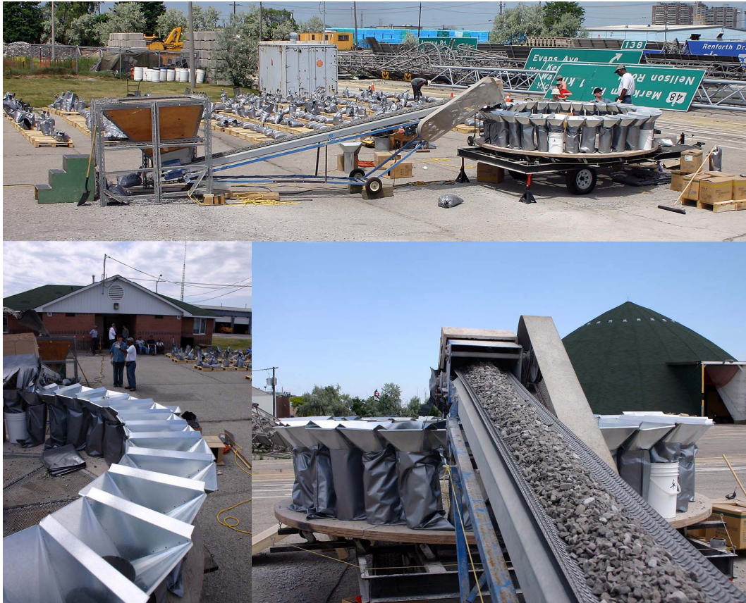
Figure 2: Spinning riffler used for preparation of samples for multi-laboratory studies of aggregate test methods.
