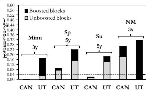
Figure 8: Expansions of boosted vs unboosted exposure blocks tested in Texas (UT) and in Ottawa (CAN).
