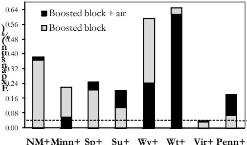
Figure 11: 4-year expansions of boosted exposure blocks, with and without air entrainment, made and tested in Texas (UT).
