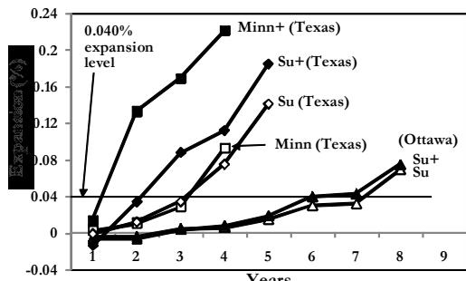
Figure 10: Expansion as a function of time for exposure blocks, boosted or unboosted, made and tested in Texas or in Ottawa.
