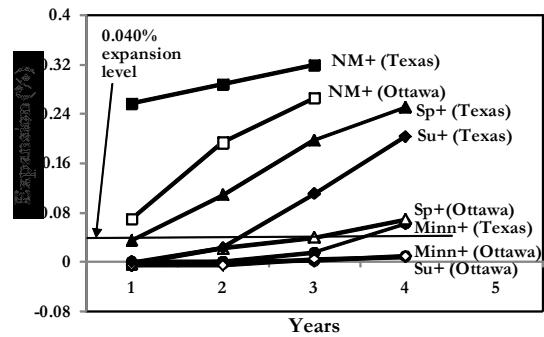
Figure 7: Expansion as a function of time for boosted exposure blocks made and tested in Texas or in Ottawa.
