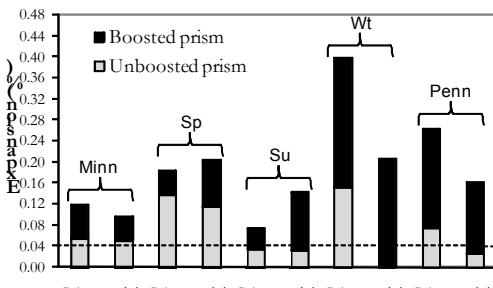
Figure 12: One-year expansion of boosted and unboosted concrete prisms incorporating the various reactive aggregates.
