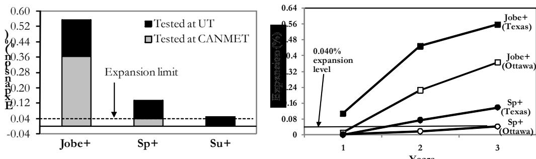
Figure 4: Three-year expansions for exposure blocks made at CANMET but tested in Texas and in Ottawa.
