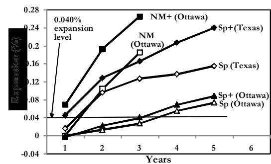
Figure 9: Expansion as a function of time for exposure blocks, boosted or unboosted, made and tested in Texas or in Ottawa.
