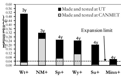
Figure 6: Three or four-year expansions of exposure blocks made and tested in Texas (UT) or in Ottawa (CANMET).
