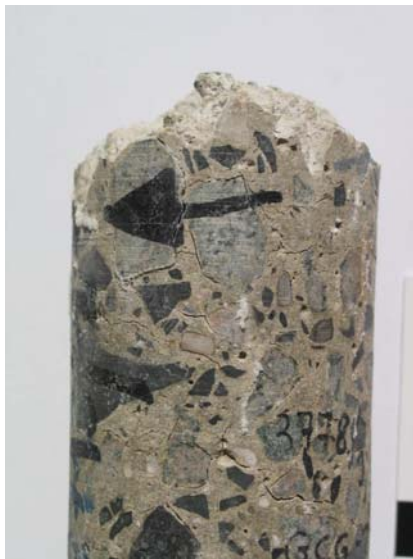
Figure 4: Bridge FH after the “GCG-DUG” test. Concrete is completely cracked (ø 50 mm).
