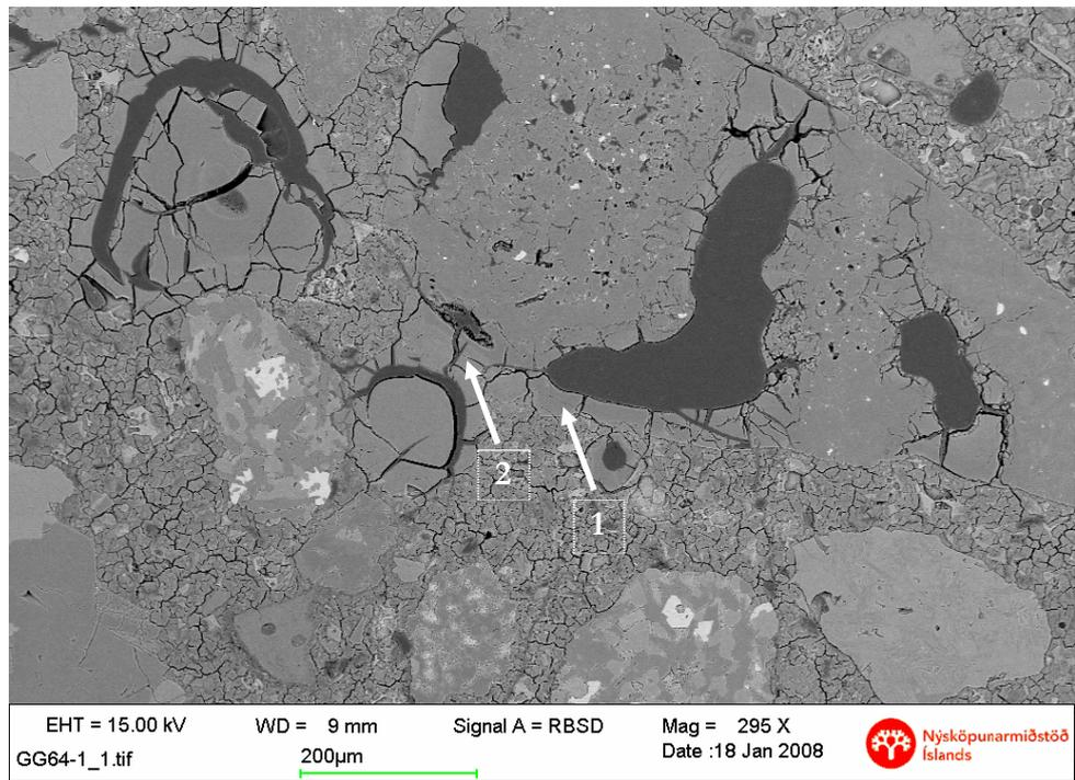
Figure 5: Alkali silica gel in a void adjacent to a basaltic aggregate. The arrows point to the areas which were analyzed.
