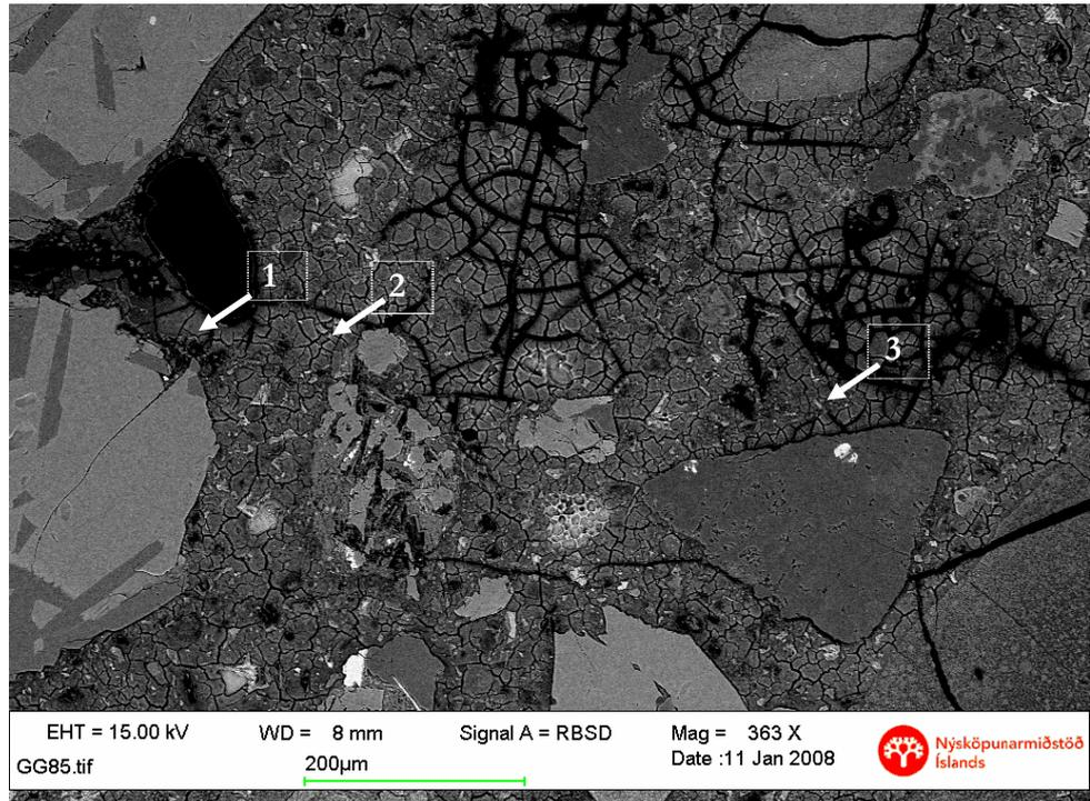
Figure 4: SEM microphotograph of alkali silica gel in shotcrete. The gel is connected to a crack. The arrows point to the areas where the composition of the gel was analyzed.
