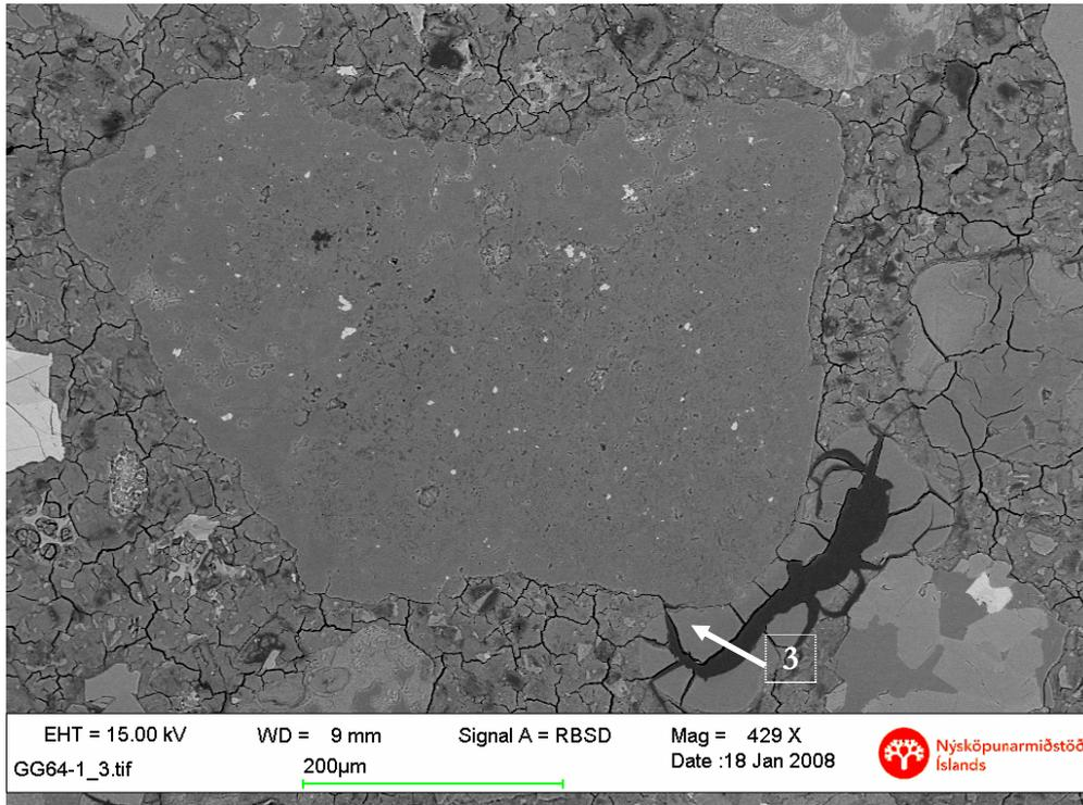
Figure 6: Alkali silica gel in void adjacent to rhyolitic aggregate. The arrow points to the area which was analyzed.
