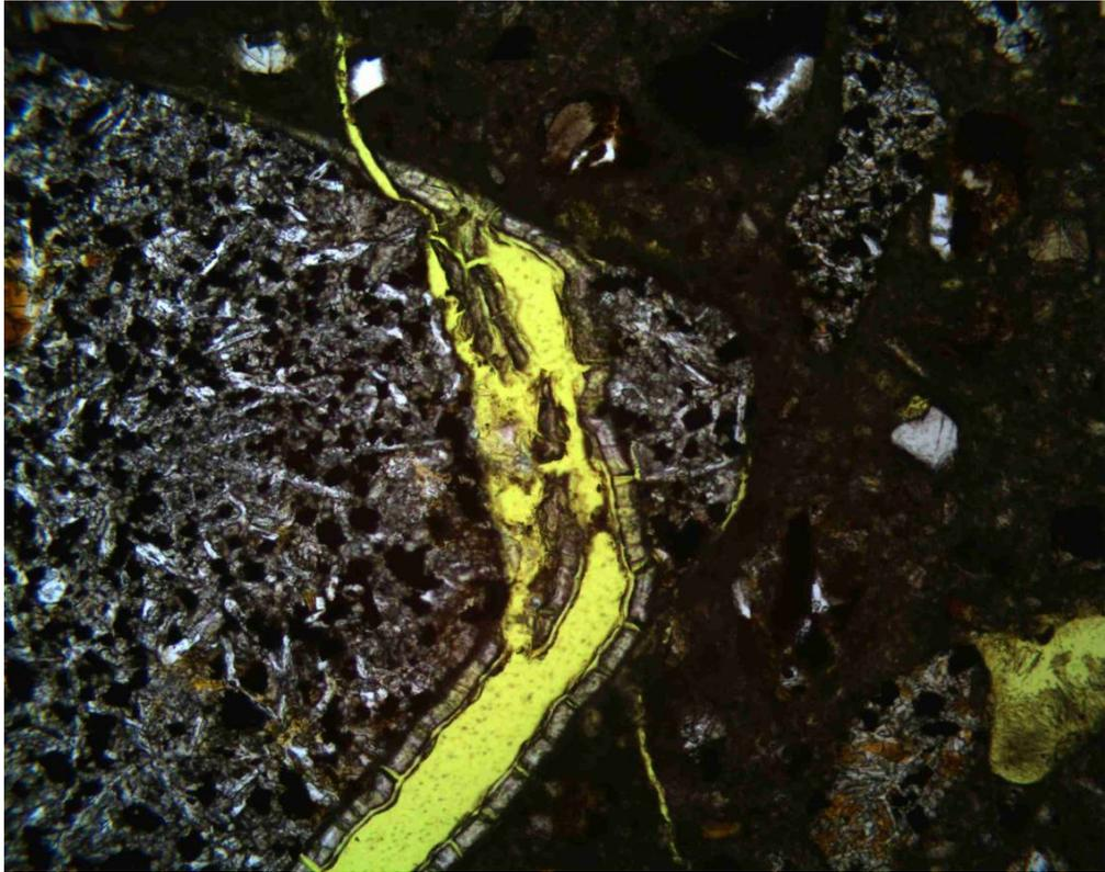
Figure 2: Photomicrograph of shotcrete showing ASR crack carrying gel in basaltic aggregate. The field of view is  $1.39 \times 0.965$ mm.
