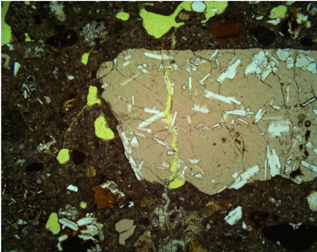
Figure 3. Photomicrograph of shotcrete showing ASR crack carrying gel in basaltic glass aggregate. The field of view is  $1.39 \times 0.965$ mm.
