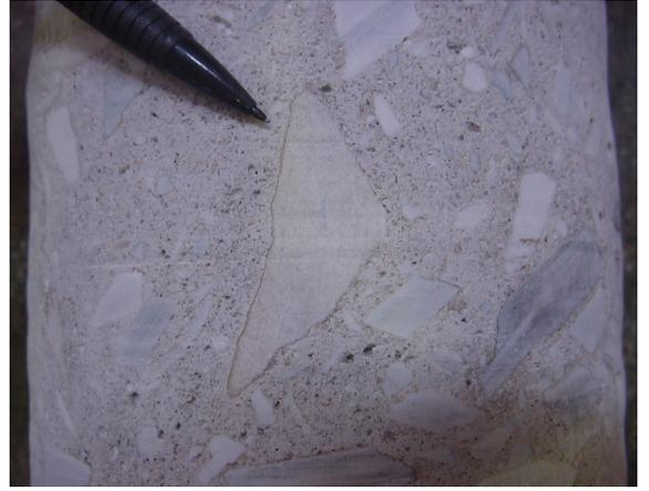
Figure 9: Dark rim around aggregate (Core 25A-US2).
