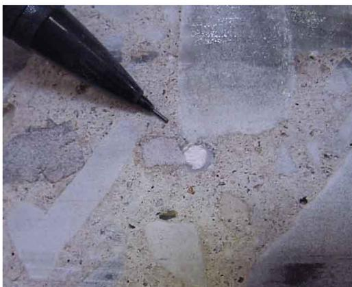
Figure 6: Void filled with white material in the interior and vitreous round the edge (Core 30A-US1).
