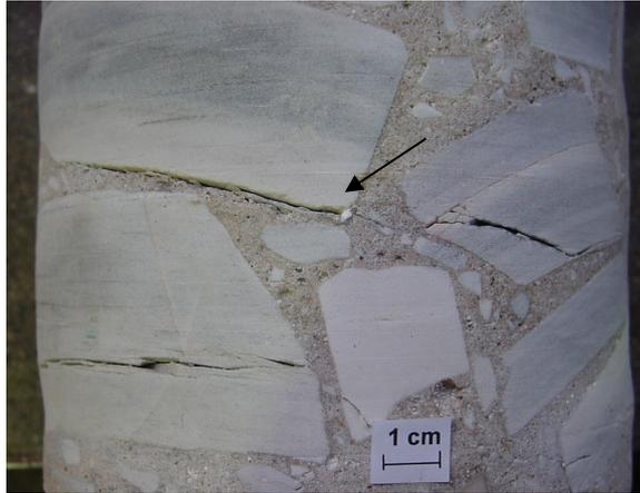
Figure 8: Cracks cutting across aggregates and white product filling in the crack (Core 12A-US2).
