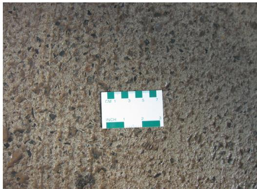
Figure 2: Exposed aggregate on part of 50% slag concrete in 2004 at 6 years due to de-icer scaling and/or abrasion.
