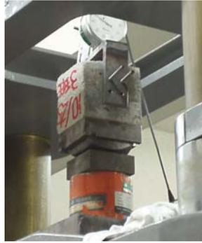
Figure 2: JSCE bond strength test.
