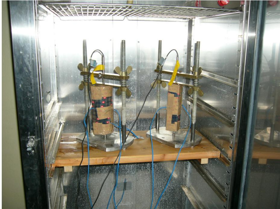
Fig. 1: Invar steel frames with LVDT's and moisture sealed specimens in freezer, left: 1/1 (Ø100/h200 mm), right: 1/4 (radius 50/h200 mm)
