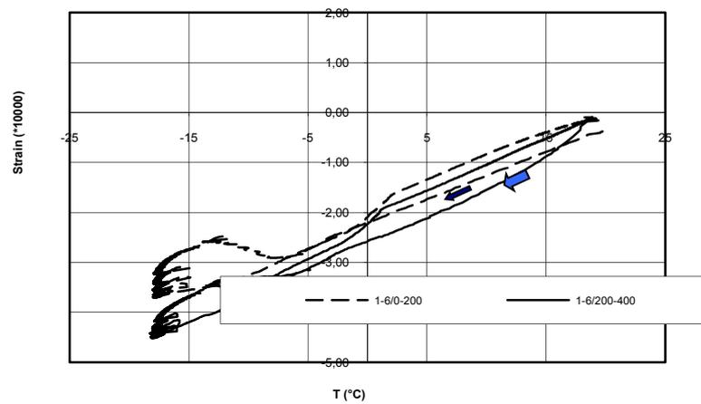
Fig. 8: Prolonged freezing period of specimen 1-6/0-200 and 1-6/200-400 at DCS=100 % with max dilation 0.1 and 0.07 ‰, respectively.
