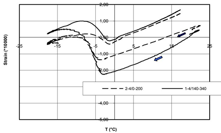
Fig. 6: Freezing dilation of specimen 2-4/0-200 and 1-4/140-340 after severe pre-drying with max dilation 0.23 ‰ at -14.5 °C and 0.48 ‰ at -14 °C, respectively
