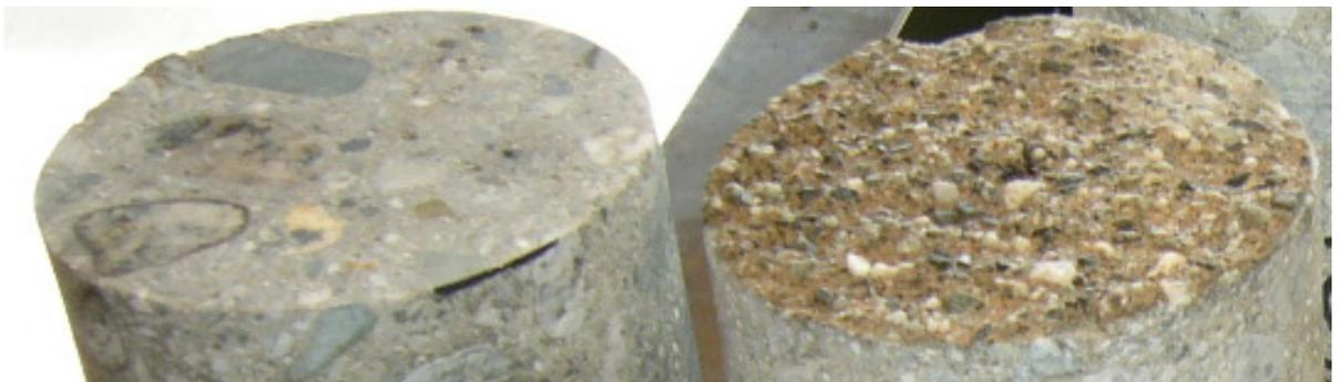
Fig.4: 100 mm diameter cores; left: sawn surface, right: horizontal dam surface with real frost scaling
