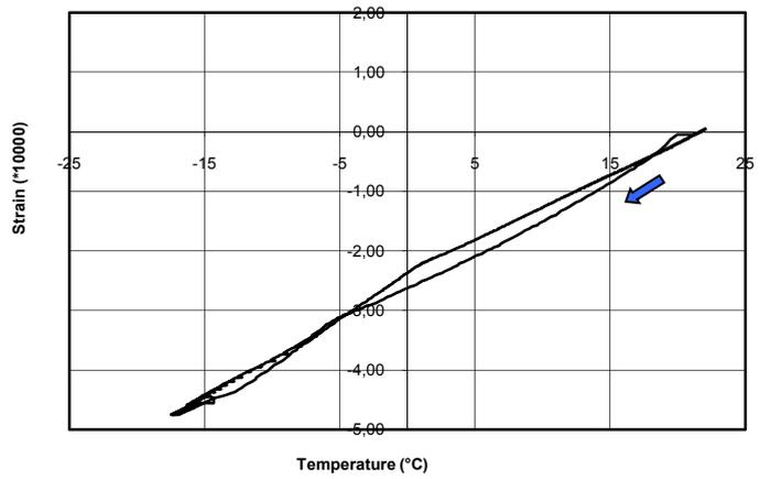
Fig. 5: Freezing dilation of specimen 1-5/200-400 at DCS=95% with max dilation 0.02 ‰ at -13 °C (left) and the same specimen further dried to DCS=92 % and re-tested giving slight contraction (right)
