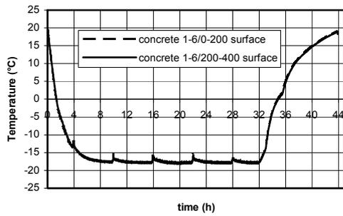
Fig.2: Concrete surface temperature vs. time; 3 h min. temperature (left) vs. 24 h prolonged freezing (right)
