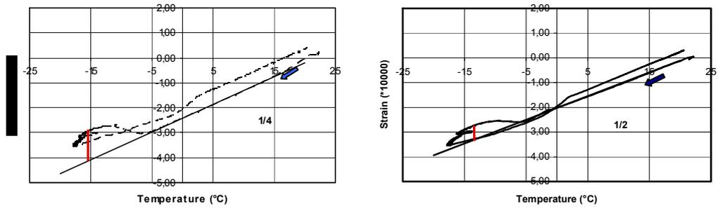
Fig. 7: Freezing dilation of specimens with different size; 1-1/200-400 (1/4): max dilation 0.12 ‰ at -16 °C (left) and 1-1/200-400 (1/2): max dilation 0.06 ‰ at -13 °C (right), both with DCS=100 %
