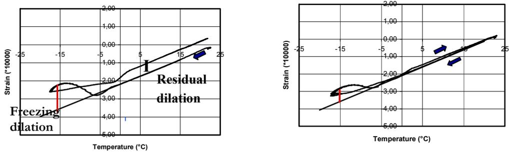
Fig.3: Freezing dilation of specimen 1-3/0-200 at DCS=100% with max dilation 0.14 ‰ at -16 °C (left) and 1-5/0-200 at DCS=97 % with max dilation 0.08 ‰ at -15 °C (right)
