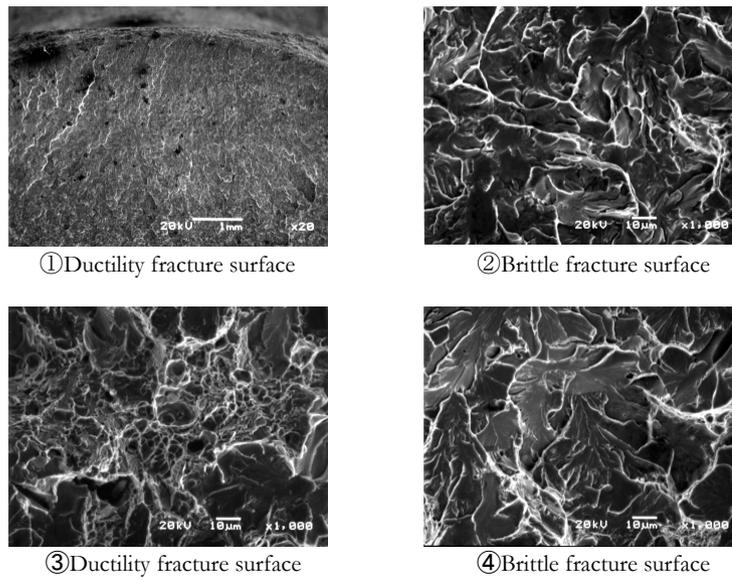
Figure 11 : SEM observation results of the fracture surface of a reinforcing bar.
