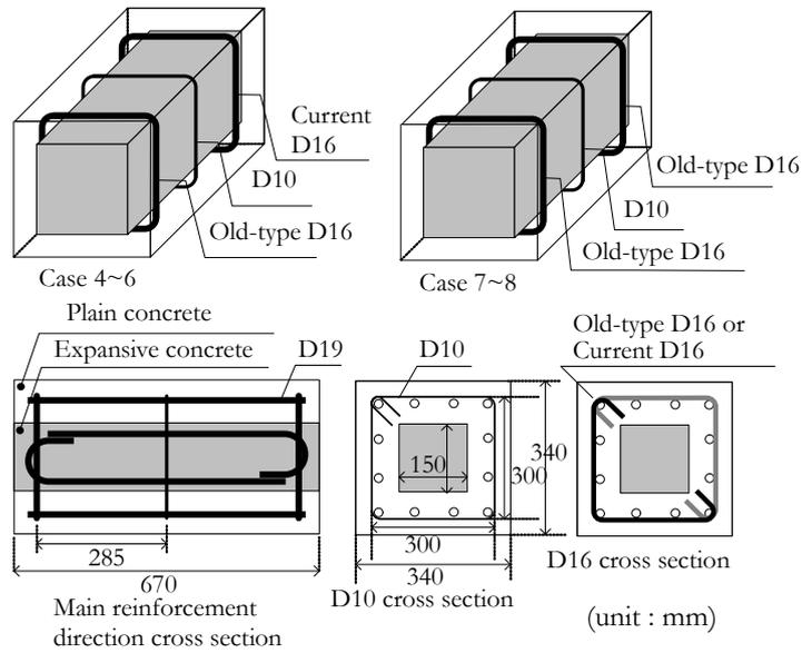
Figure 2 : Shape and dimensions of test specimens.
