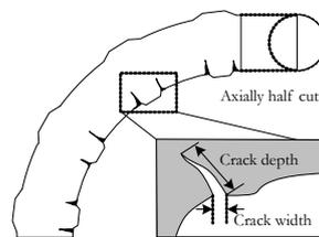
Figure 3 : Method for measuring cracks.
