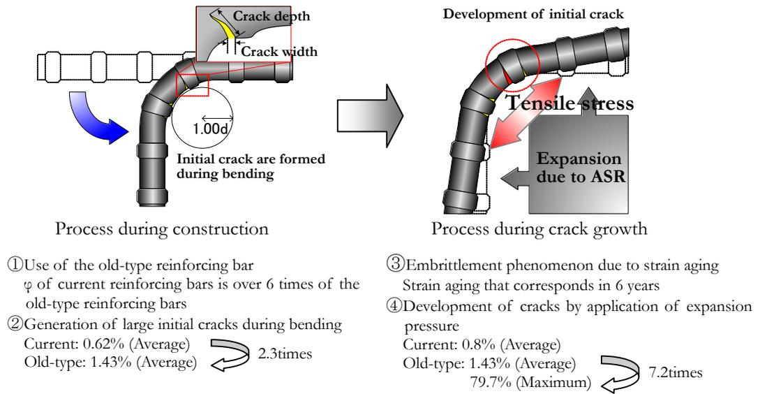
Figure 12 : Rupture mechanism of reinforcing bar.
