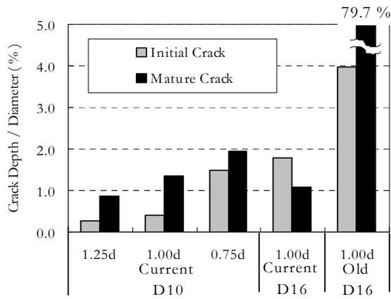
Figure 6 : Comparison of the maximum crack depths.
