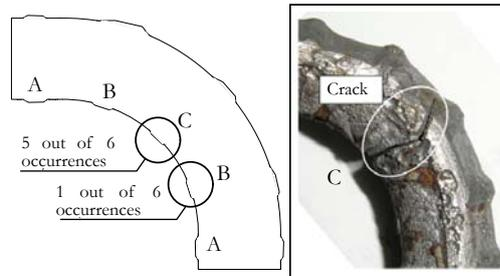
Figure 9 : Position of Cracks.
