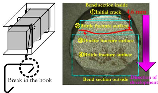
Figure 10 : Rupture of a reinforcing bar.
