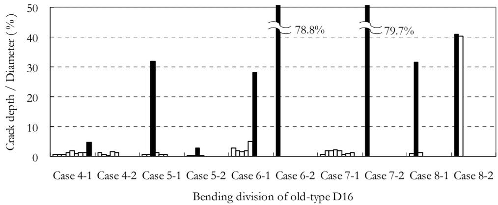
Figure 8 : Comparison of depth of mature cracks in old-type reinforcing bar.
