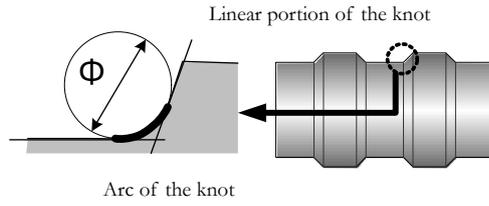
Figure 4 : Method for measuring knot shape.
