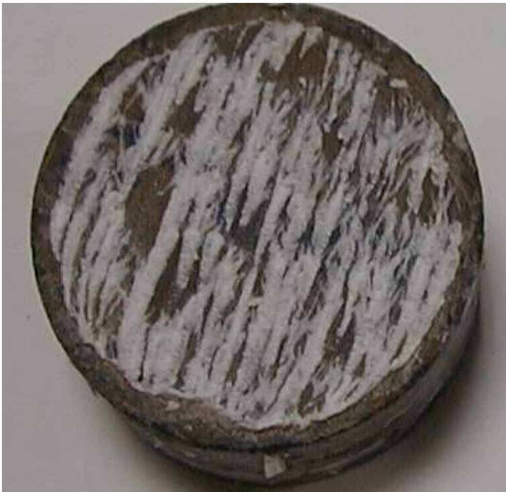
Figure 2: White crystals of \text{CaCO}_3 appear on the surface of 5cm height specimen in the cathode after the RLMT test
