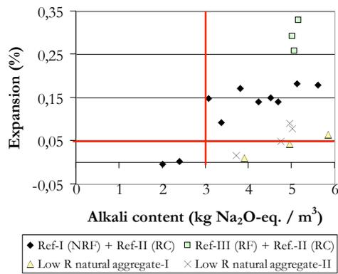
Figure 10: Expansion versus alkali content for four Norwegian aggregate types after one year of exposure (F=Fine and C=Coarse aggregate). The lines drawn at 3.0 kg Na<sub>2</sub>O eq. /m<sup>3</sup> and 0.05 %, respectively, represent Norwegian critical limits.
