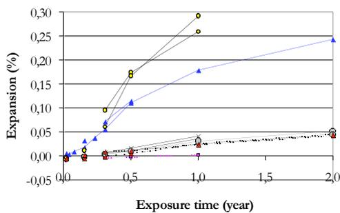
Figure 4: Expansion versus exposure time for six parallel concrete mixes.
