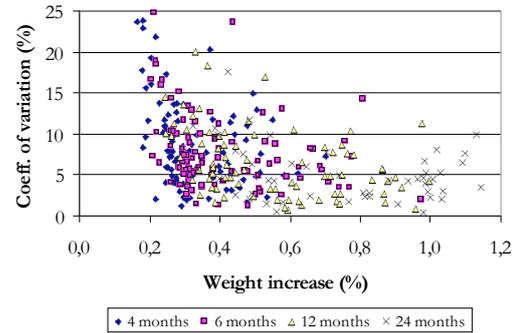
Figure 3: Coefficients of variation (c.o.v) for the weight increases of the three prisms within one test series (about 100 SINTEF test series).
