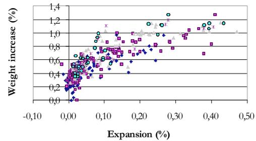
Figure 11: Weight increase versus expansion (at the ages 0.5, 1, 2, 3 and 4 years, respectively) for the 144 performance test series.
