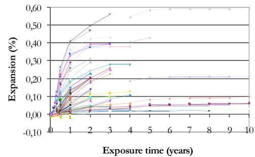
Figure 5: Expansion versus exposure time for 144 performance test series.
