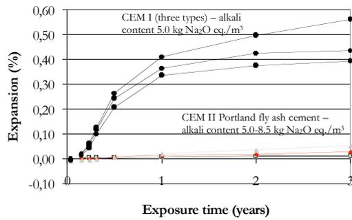
Figure 8: Expansion versus exposure time for 6 binders tested with the aggregate combination Ref-I (NR-fine) + Ref-II (R-coarse) -see Table 1. The CEM II Portland - fly ash cement contains 20 % PFA (80 kg/m<sup>3</sup>).
