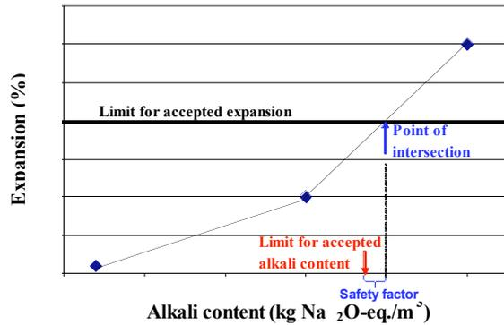
Fig. 1: Principle diagram for determination of acceptance limit for alkali content.
