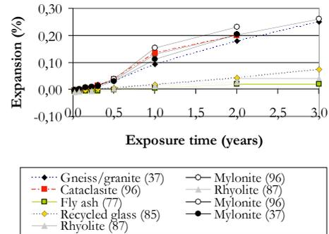
Figure 9: Expansion versus exposure time for concretes containing different fillers (0-0.125 m) and a reactive mylonite aggregate [19]. The number in () is kg filler pr m<sup>3</sup>. The alkali content in all mixes was about 5.0 kg Na<sub>2</sub>O eq. /m<sup>3</sup>
