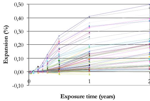
Figure 6: Expansion versus exposure time (up to two years) for 144 performance test series.
