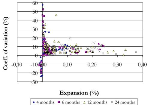
Figure 2: Coefficients of variation (c.o.v) for the expansions of the three prisms within one test series (about 100 SINTEF test series).
