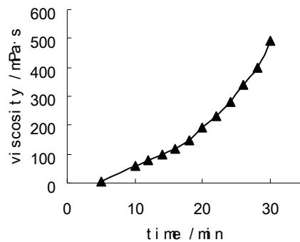
Figure 1: Relation of viscosity with preparation time.
