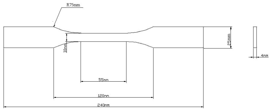
Figure 3: Dimensions of sample for tension strength testing.
