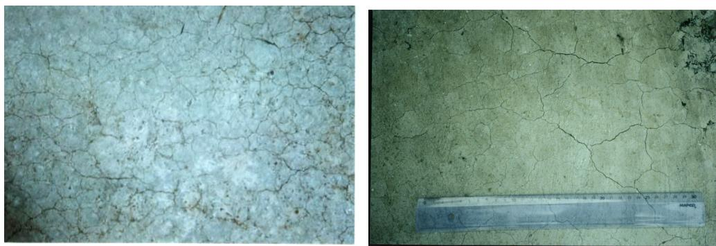
Figure 9: Cracking concrete prepared outside the lab.
