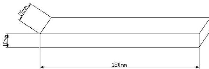
Figure 2: Dimensions of sample for bending strength testing.
