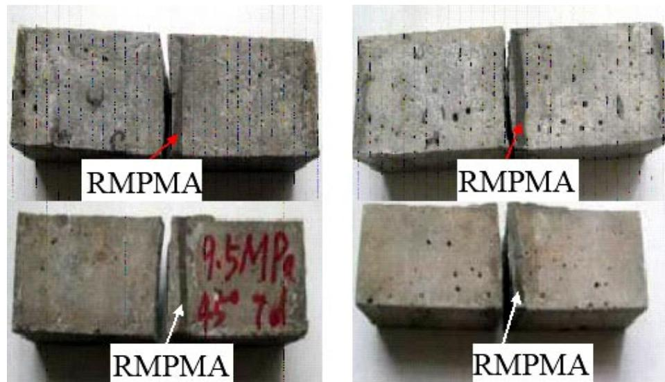
Figure 7: Photos of broken bonded mortar bars.
