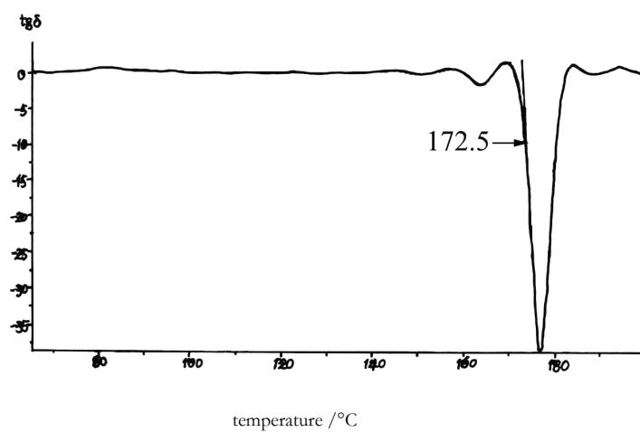
Figure 6: The Tg testing curve of RMPMA.
