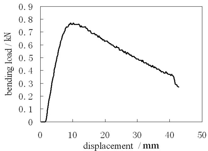
Figure 4: Relationship between bending load and displacement.
