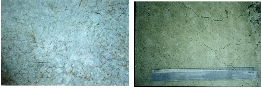
Figure 9: Cracking concrete prepared outside the lab.
