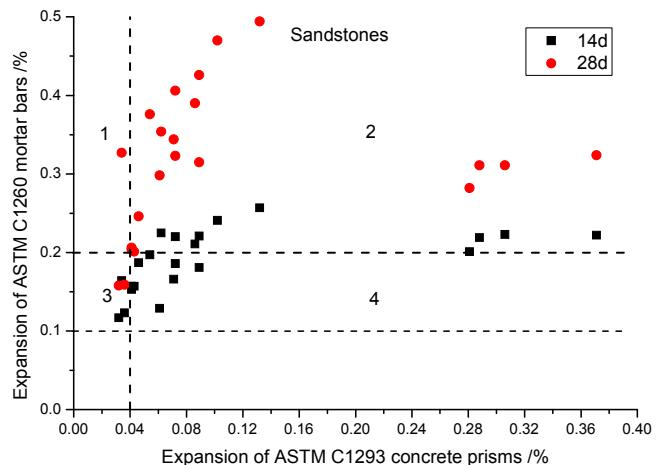
Figure 7: Correlation between expansions of ASTM C1260 accelerated mortar bars and ASTM C1293 concrete for sandstones
