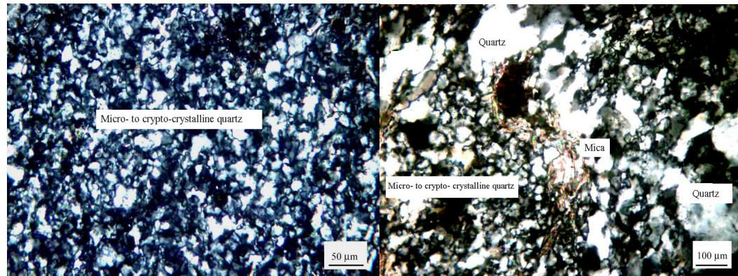
Figure 4: Micro- to crypto- crystalline quartz in chert (left) and lithoclast (right) in sands
