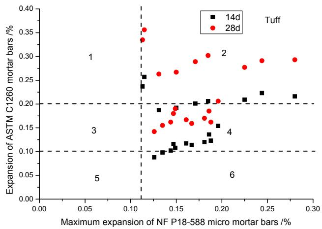
Figure 9: Relationship between the maximum expansion of NF P18-588 micro-mortar bars and expansion of ASTM C1260 accelerated mortar bars for tuffs
