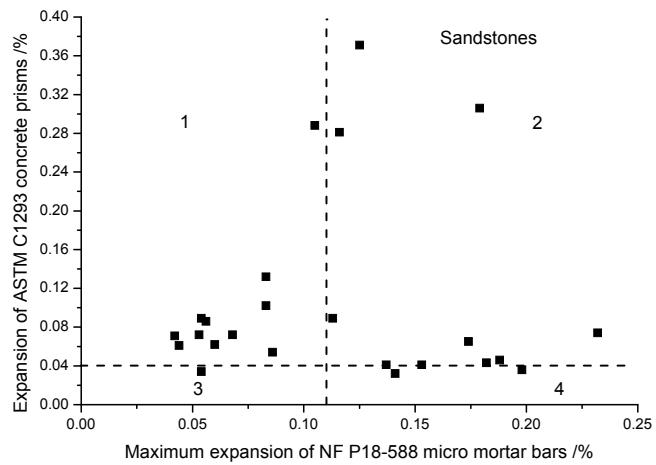
Figure 6: Relationship between the maximum expansion of NF P18-588 micro-mortar bars and expansion of ASTM C1293 concrete prisms for sandstones
