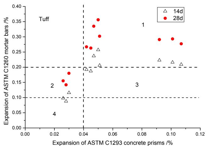
Figure 11: Relationship between expansions of ASTM C1260 accelerated mortar bars and ASTM C1293 concrete prisms for tuffs
