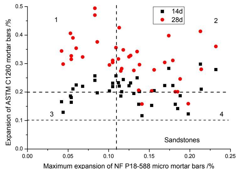
Figure 5: The maximum expansion of NF P18-588 micro-mortar bars vs expansion of ASTM C1260 mortar bars for sandstones
