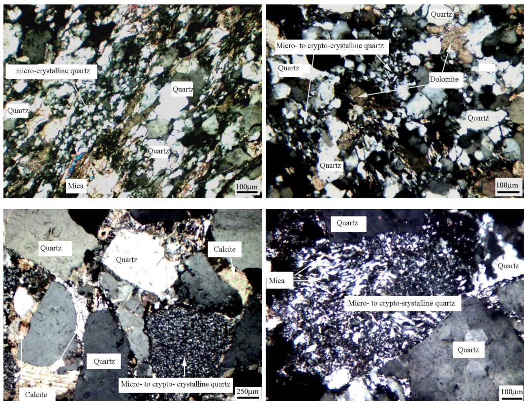
Figure 1: Typical micrructures of sandstones
