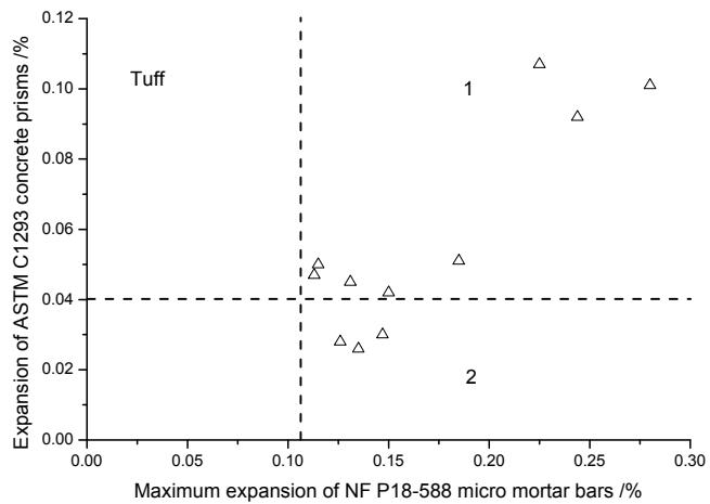
Figure 10: The maximum expansion of NF P18-588 micro-mortar bars vs expansion of ASTM C1293 concrete prisms for tuffs
