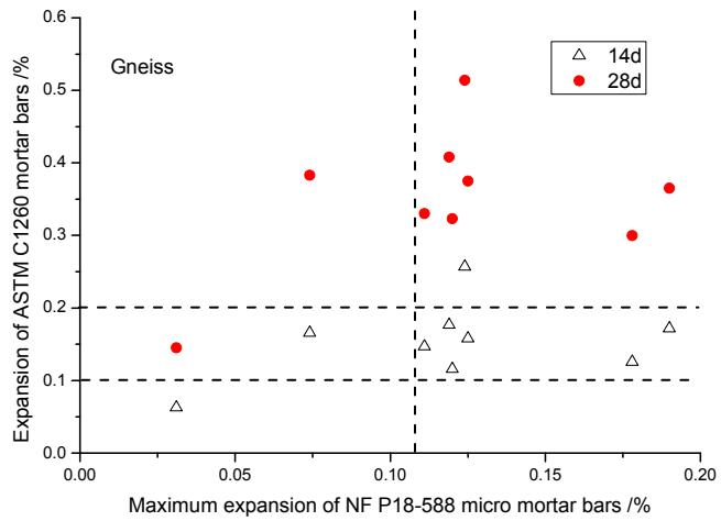
Fig 12: Relationship between the maximum expansion of NF P18-588 micro-mortar bars and expansion of ASTM C1260 accelerated mortar bars for gneisses
