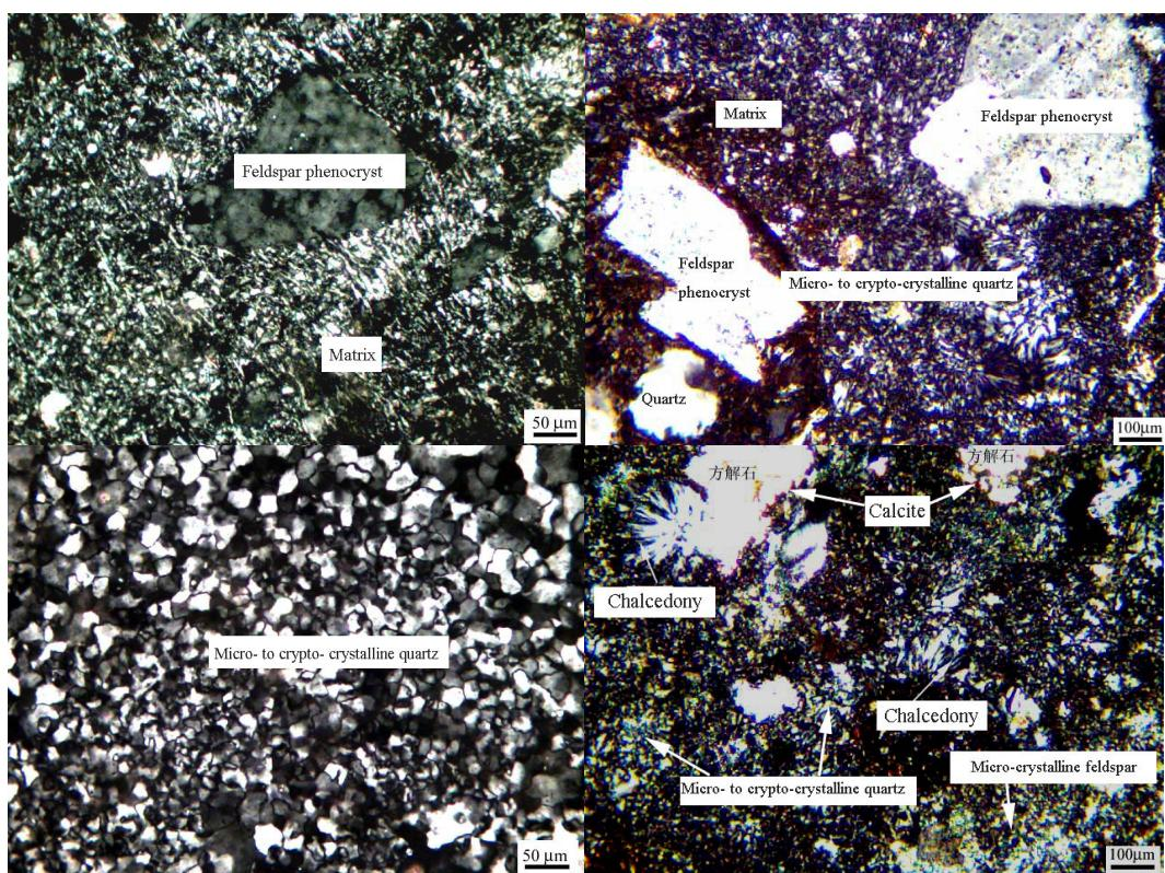
Figure 2: Typical microstructures of tuffs
