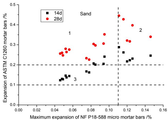
Figure 14: Relationship between the maximum expansion of NF P18-588 micro-mortar bars and expansion of ASTM C1260 accelerated mortar bars for sands
