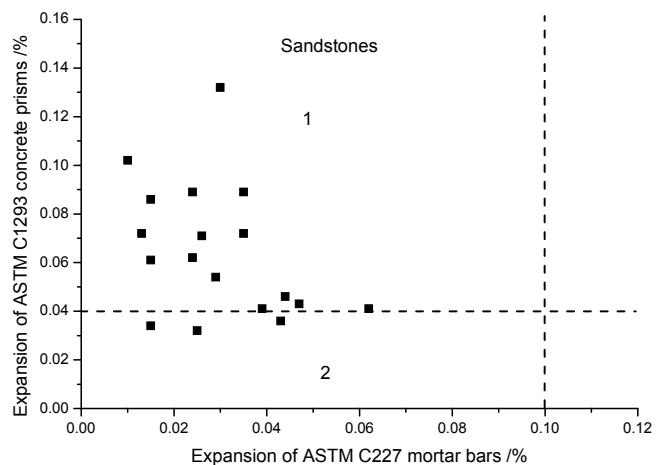
Figure 8: Correlation between expansions of ASTM C227 mortar bars and ASTM C1293 concrete prisms for sandstones
