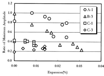
Figure 10: Correlations between the expansion and the ratios of maximum amplitude of the sampling cores
