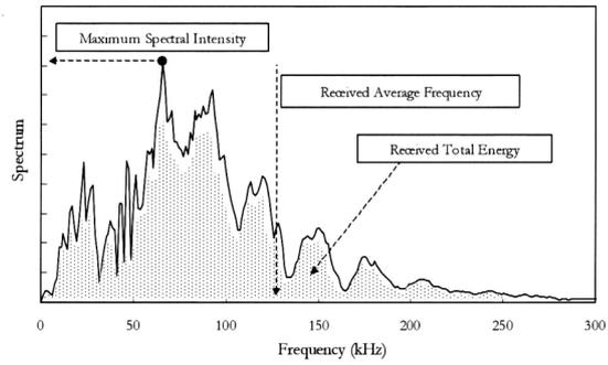
Figure 3: ultrasonic propagation characteristics estimated from a frequency distribution
