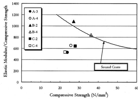
Figure 13: Relations between the ratio of elasticity modulus to compressive strength and compressive strength of the sampling cores
