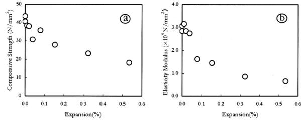
Figure 5: Correlations between the expansion and the compressive strength, the elasticity modulus
