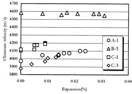
Figure 9: Correlations between the expansion and the ultrasonic velocities of the sampling cores
