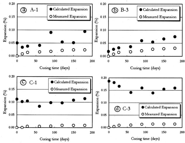
Figure 12: Comparisons between the calculated expansion and the measured expansion
