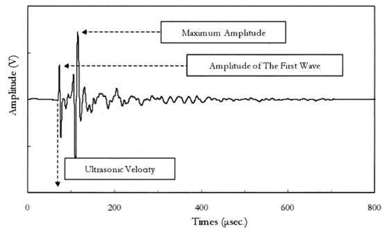
Figure 2: ultrasonic propagation characteristics estimated from a receiving wave
