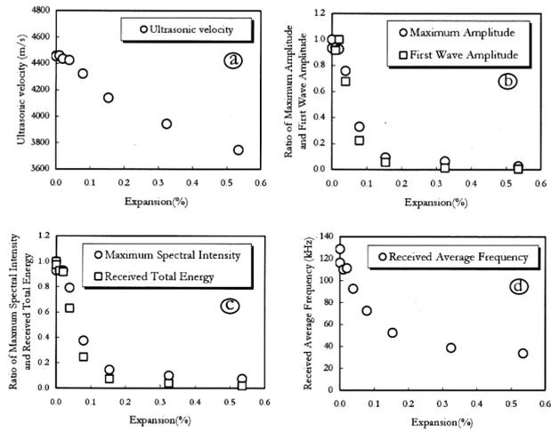
Figure 4: Correlations between the expansion and the ultrasonic propagation characteristics (the core specimens cut into 200 mm)
