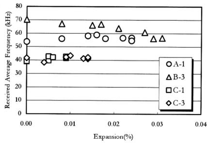
Figure 11: Correlations between the expansion and the received average frequencies of the sampling cores
