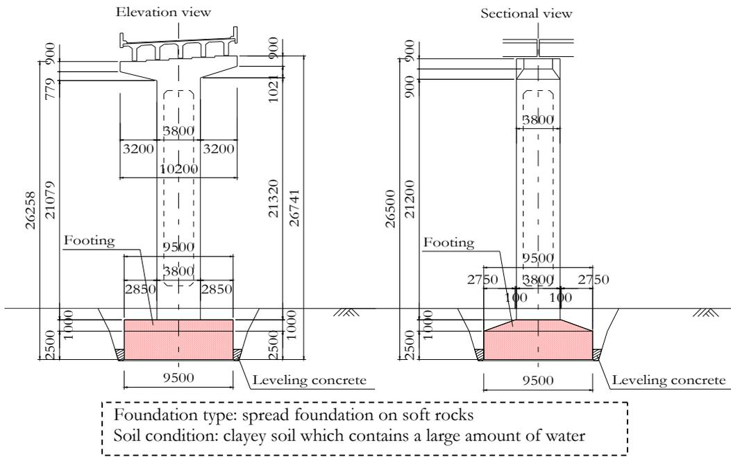
Figure 3: General drawing of the bridge pier.
