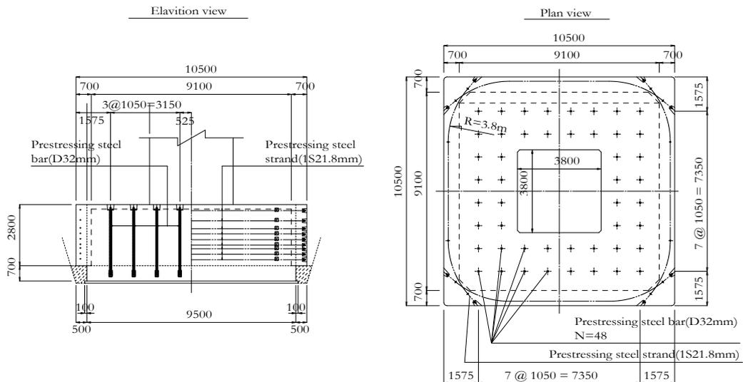
Figure 12: Layout of prestressing steel.
