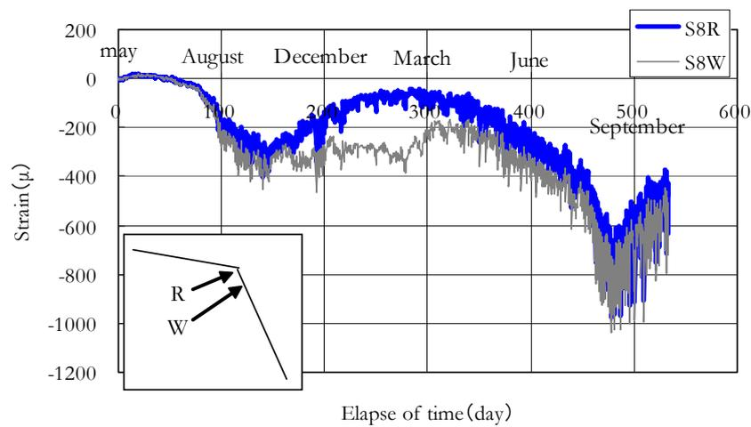
Figure 20: Change over time in strain in steel bar.
