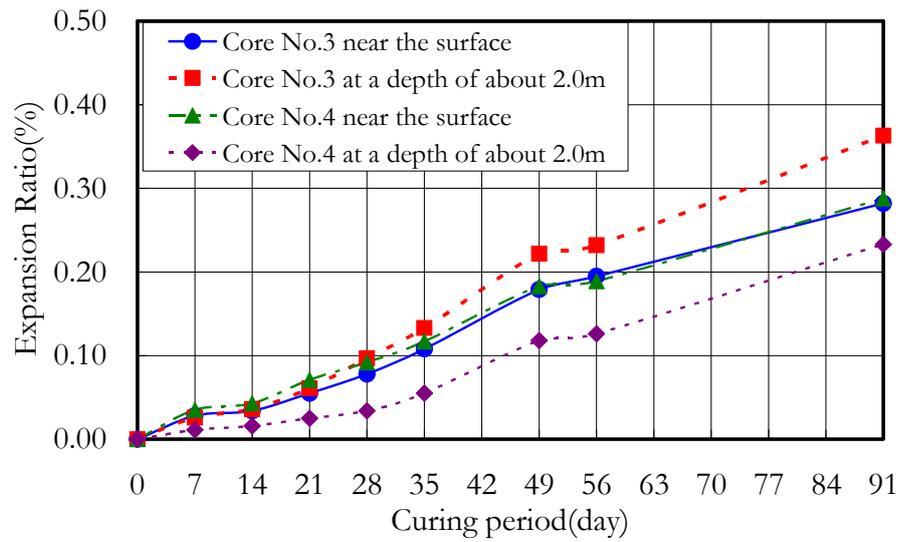
Figure 10: Results of accelerated curing test (immersed in  $50\pm 2^\circ\text{C}$  saturated NaCl solution).
