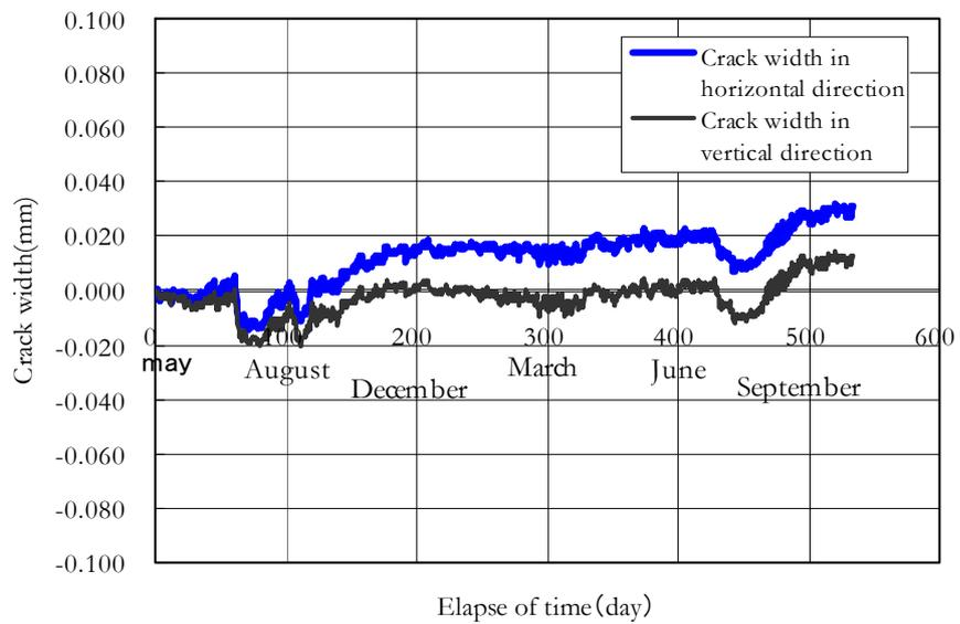
Figure 17: Change over time in crack width.
