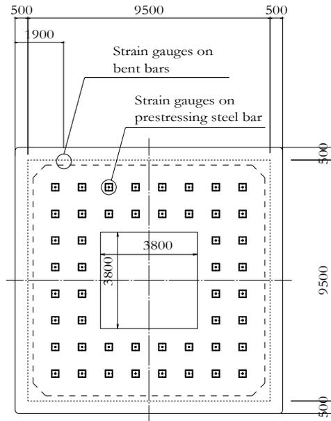
Figure 18: Location of strain gauges on prestressing steel bars and bent bars.
