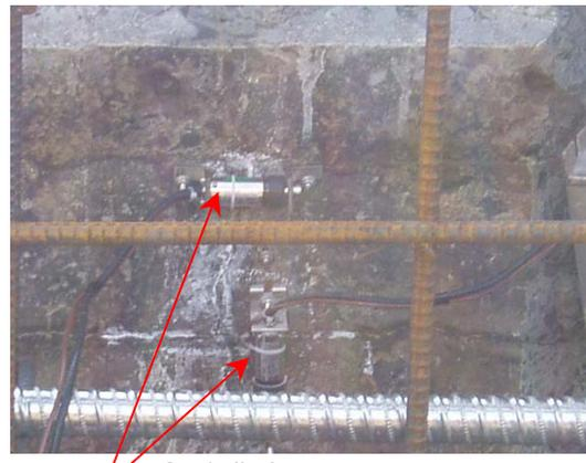
Crack displacement gauge
