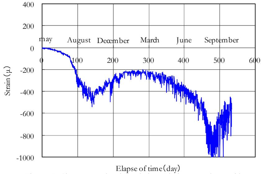
Figure 19: Change over time in strain in vertical prestressing steel bar.
