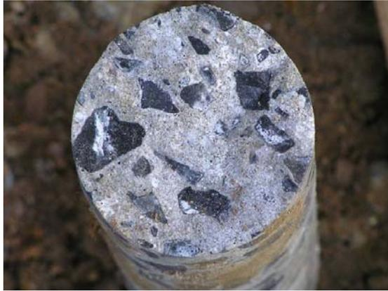
Figure 7: Cross-sectional view of a core sample (ø100 mm).
