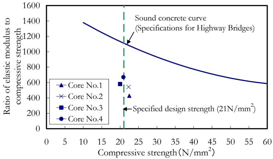
Figure 8: Relationship between the concrete compressive strength and the ratio of the elastic modulus to compressive strength ( $E_c/f_c$ ).
