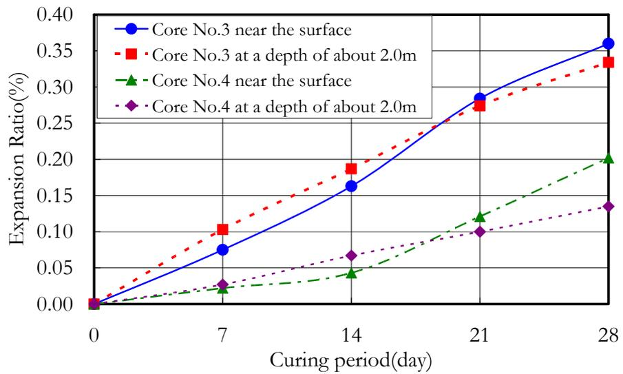
Figure 9: Results of accelerated curing test (immersed in  $80\pm 2^\circ\text{C}$  1N-NaOH solution).
