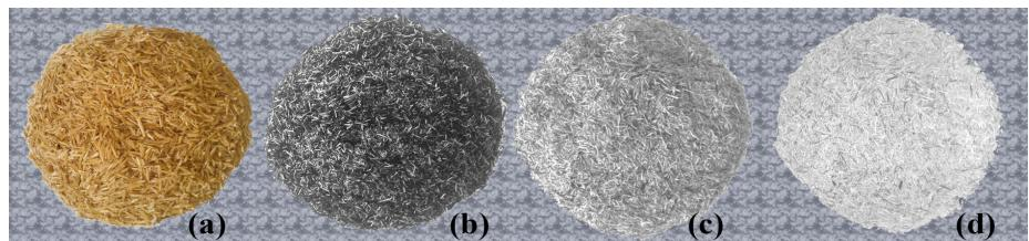
Figure 3: (a) rice husk (b) high carbon RHA (c) optimum RHA (d) RHA with crystalline silica.
