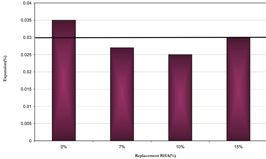
Fig 9: Expansion of concrete prisms (RILEM AAR-4) at 6 months.
