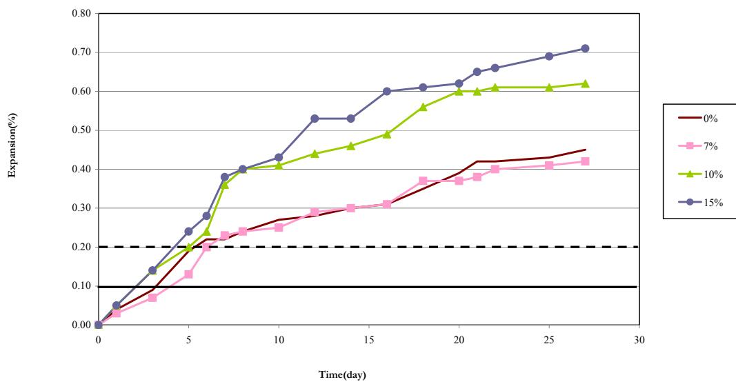
Fig 6: Effect of RHA content on expansion of mortar bars (ASTM C 1260).
