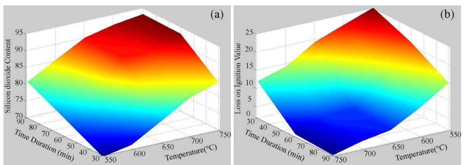
Figure 2: Estimated variation of (a) SiO<sub>2</sub> and (b) LOI VS. temperature and time duration.
