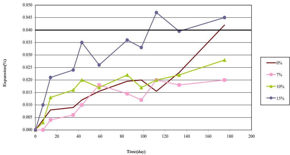
Fig 8: Effect of RHA content on expansion of concrete prism (ASTM C 1293).
