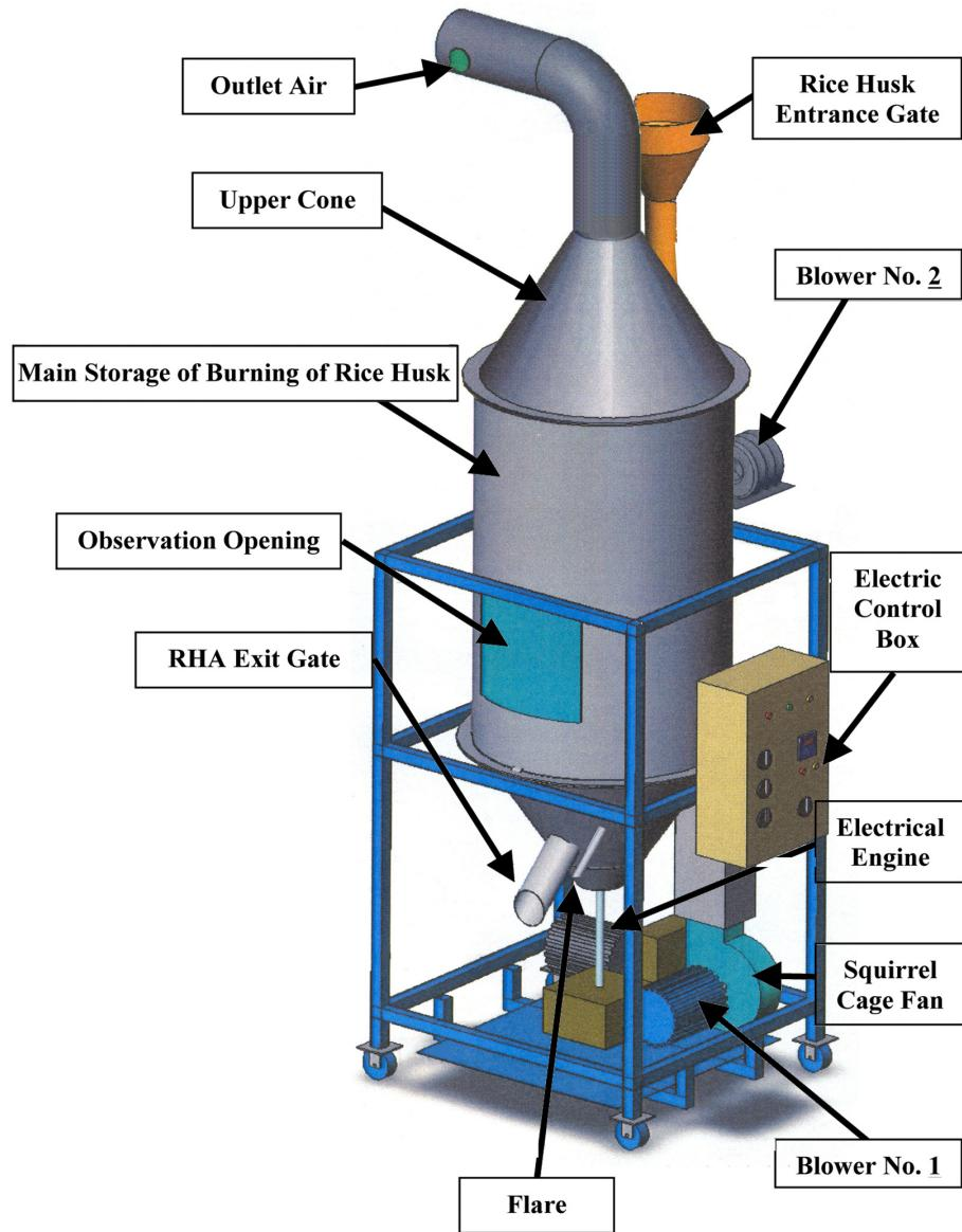
Figure 1: schematic shape of rice husk ash furnace.
