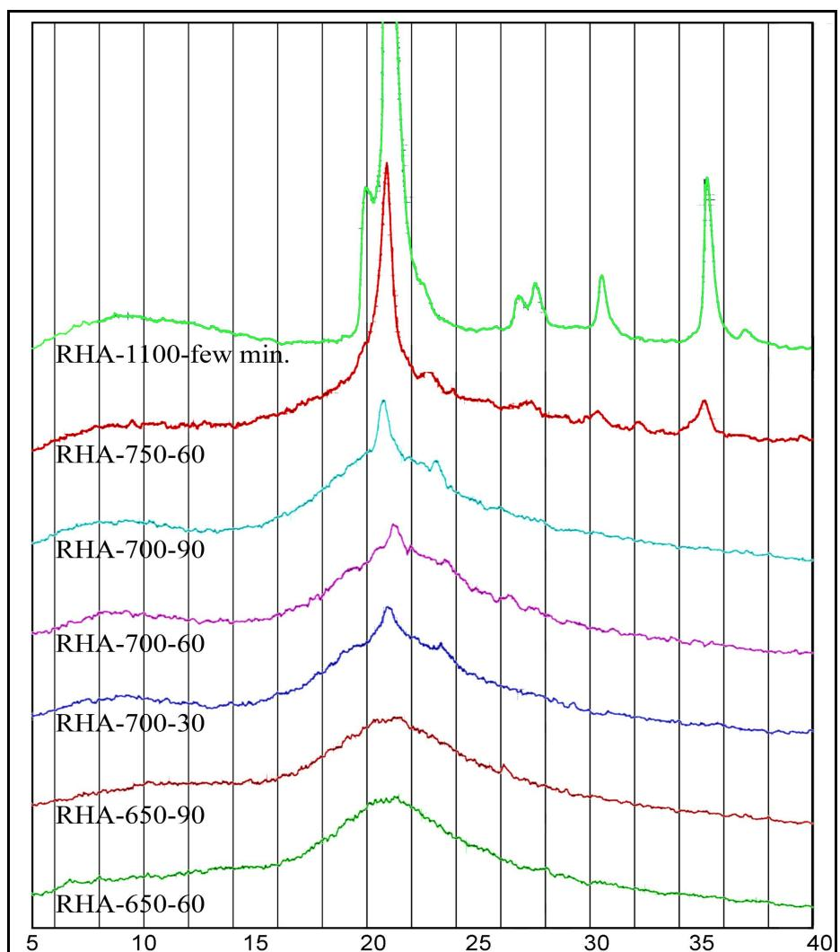
Figure 4: Results of XRD on rice husk ash samples and cement.
