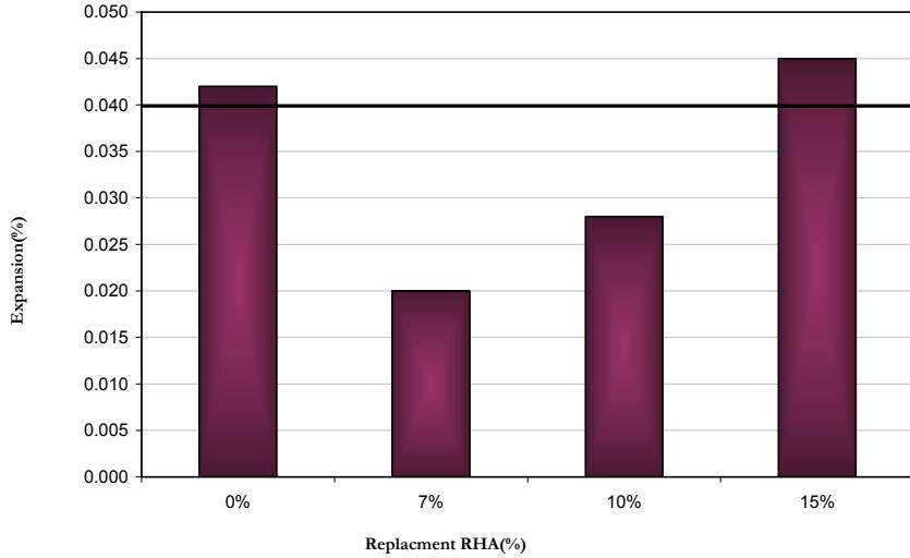
Fig 7: Expansion of concrete prisms (ASTM C 1293) at 175 days.
