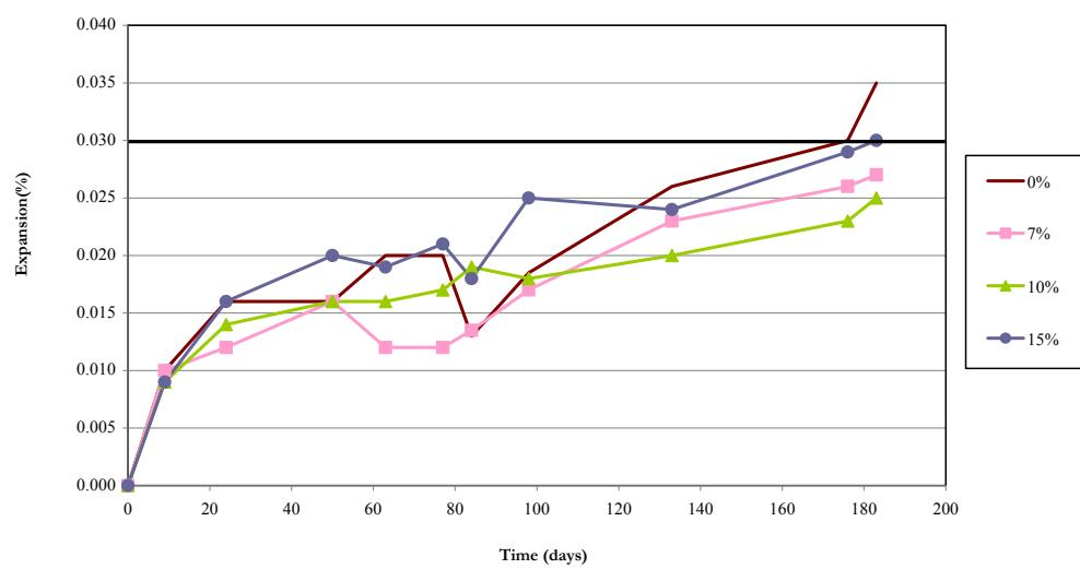
Fig 10: Effect of RHA content on expansion of concrete prism (RILEM AAR-4).
