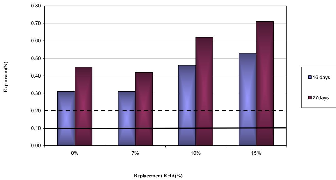
Fig 5: Expansion of mortar bars at 16 and 27 days.
