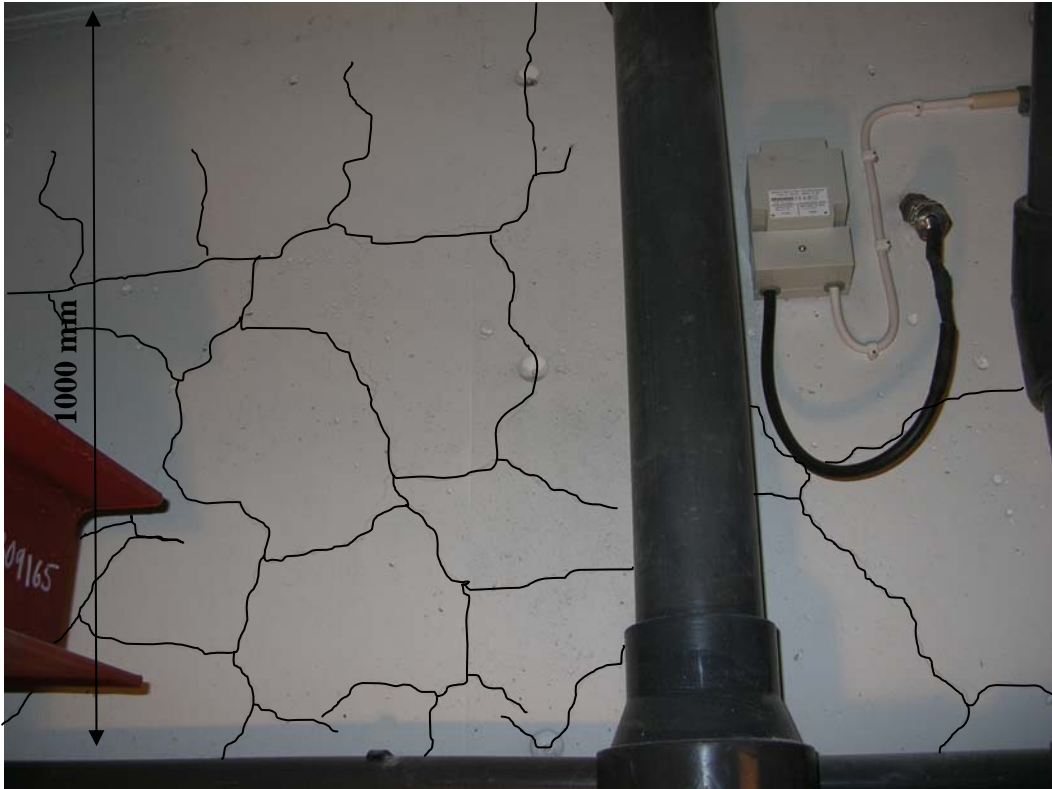
Figure 1: Map cracking on the outside face of the pool wall. Note that the cracks are intensified by drawings on the photo.
