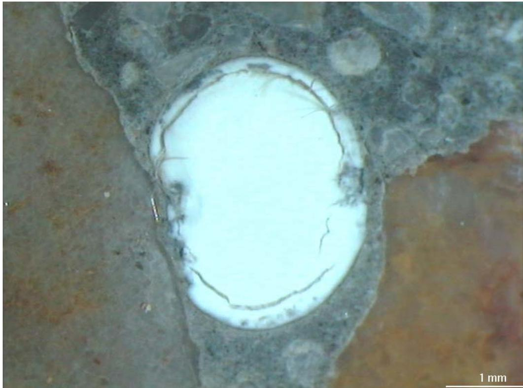
Figure 3 – View of a polished section of concrete showing a white deposit filling an air void.
