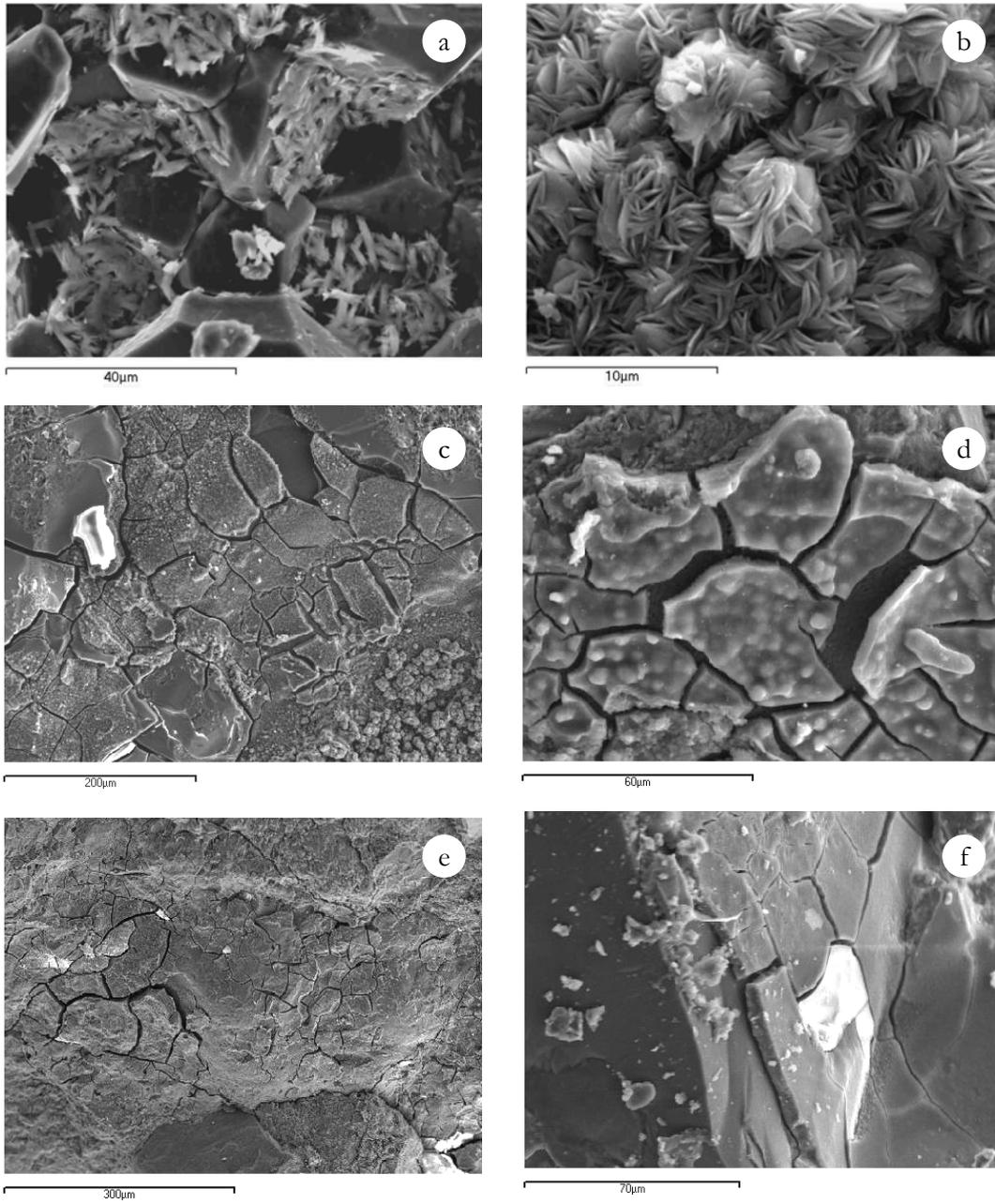
Figure 5 – SEI images showing various forms of ASR products (◻): (a) lamellar crystals in a quartzite grain, (b) rosette-like crystals, (c-d) concomitance of bump-shaped gel and botryoidal products, (e-f) smooth gel.
