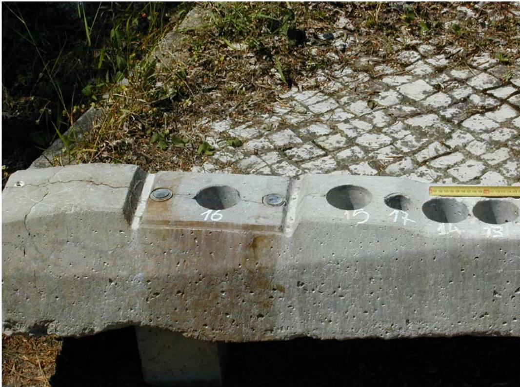
Figure 2 – View of the concrete sleeper A type after core drilling.
