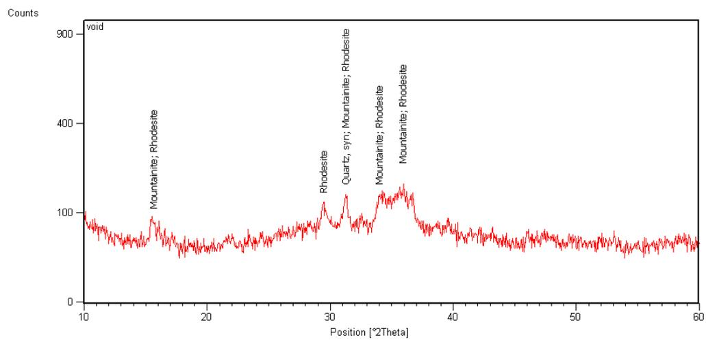
Figure 4 – XRD pattern of a white material removed from a concrete void.
