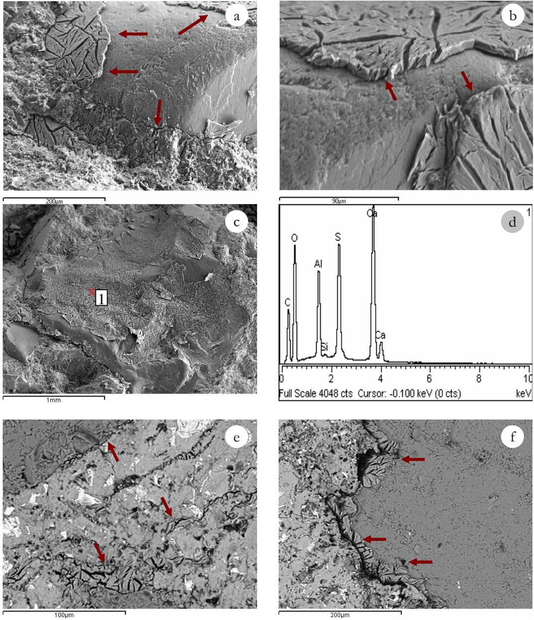
Figure 6 – Different aspects of ettringite formation in the cracked sleepers A and B types: (a-c) SEI images of compressed ettringite on aggregate particles, (d) EDX spectra of ettringite marked in Figure 2c, (e-f) BSE images of compressed ettringite in the paste and around aggregate particles.
