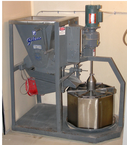
Figure 1: Rotary sample divider with a 50 liter hopper and an outlet that can take maximum 50 mm big particles.
