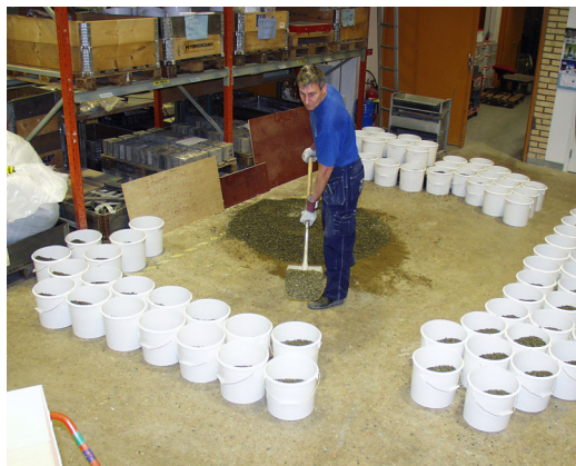
Figure 2: Fractional shovelling, in accordance with EN 932-2.
