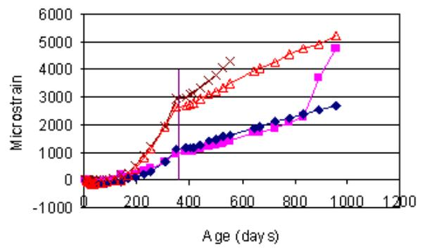
Pile 14- Steam curing, half-immersed in salt solution, Hr aggregate, 5% SO<sub>3</sub>
