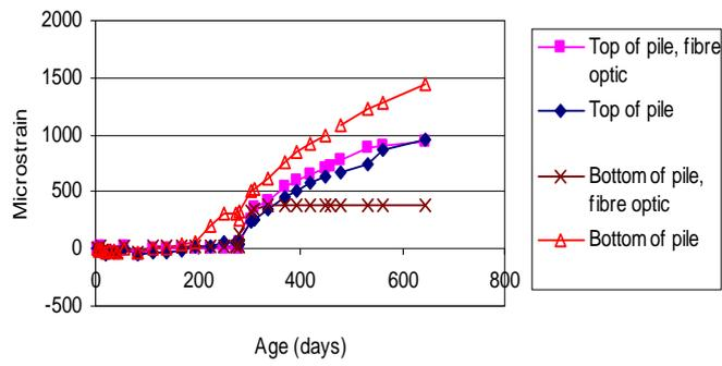
Figure 15: Comparison of readings of fibre optic and foil concrete gauges in Pile 12.
