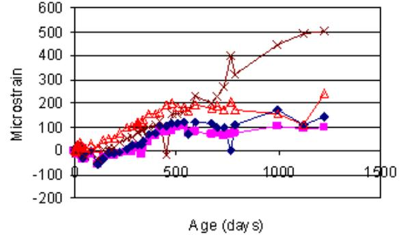
Steam curing, half-immersed in salt solution, Nr aggregate
