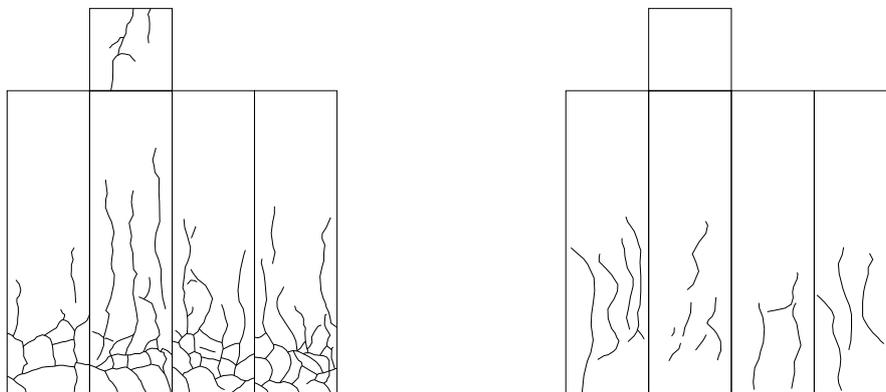
Figure 6: Cracking developed in pile 11 at two years (left) and in pile 14 at one year (right).
