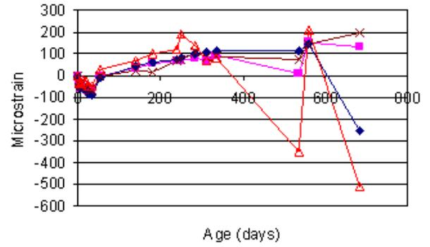
Pile 16- Normal curing, half-immersed in water, Nr aggregate, 5% SO<sub>3</sub>
