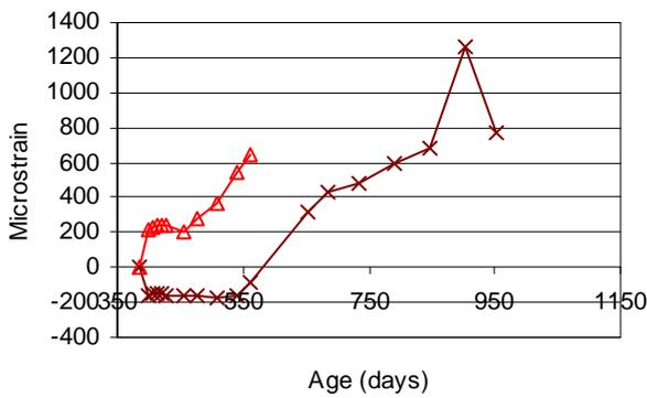
Highly reactive concrete, steam curing, half-immersed in water.
