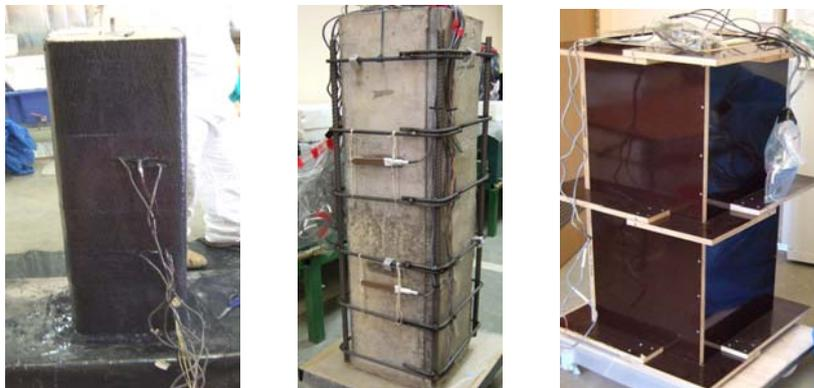
Figure 7: Views of model piles after repair with CFRP (left); fitted with reinforcement (centre) and after fitting mould for casting concrete jacket (right).
