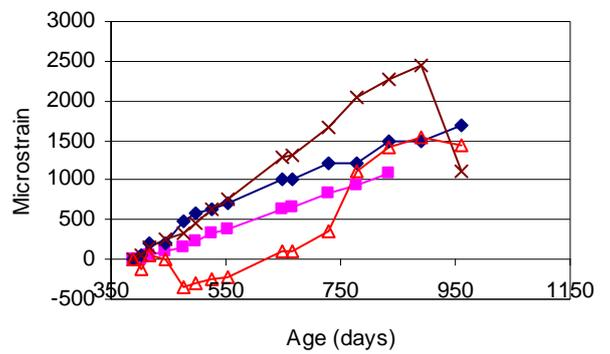
Highly reactive concrete, steam curing, half-immersed in salt solution. Highly reactive aggregate, high sulphate.
