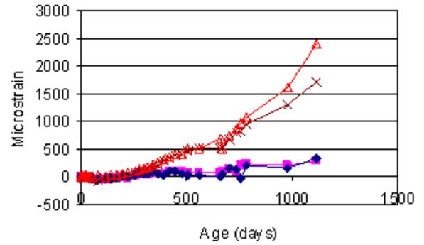
Steam curing, half-immersed in salt solution, Lr aggregate
