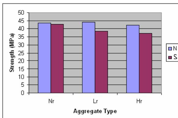
Figure 8: compressive strength at 28 days.
