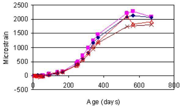
Pile 15- Steam curing, half-immersed in water, Nr aggregate, 5% SO<sub>3</sub>
