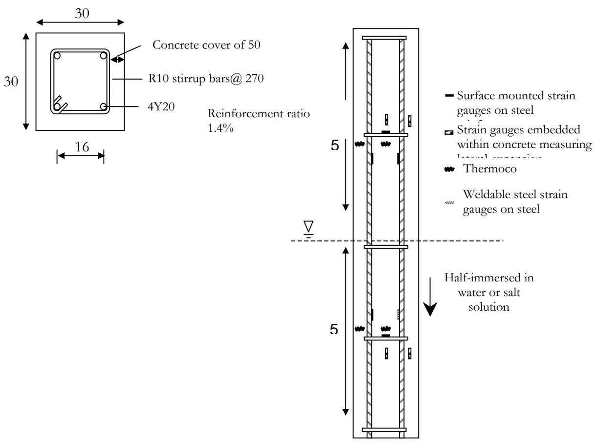
Figure 2: Cross section and reinforcement details of pile specimen.
