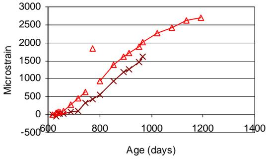
Steam curing, half-immersed in salt solution
