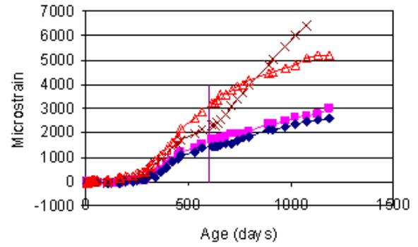
Pile 11- Steam curing, half-immersed in salt solution. Hr aggregate, 2.6% SO<sub>3</sub>
