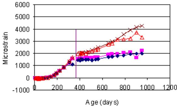
Pile 13- Steam curing, half-immersed in water, Hr aggregate, 5% SO<sub>3</sub>
