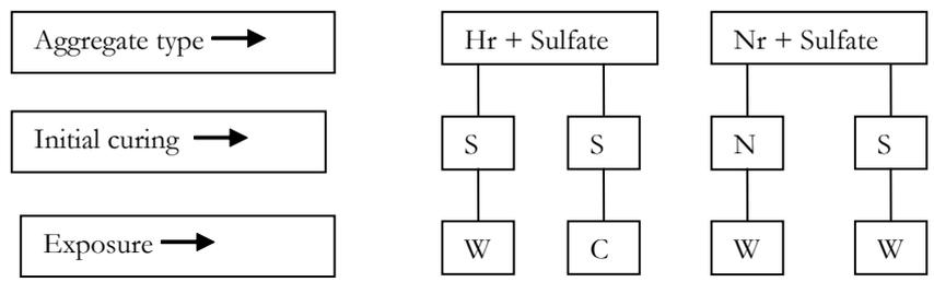
Figure 1b: Combination of variables in the second set of four piles (13-16).
