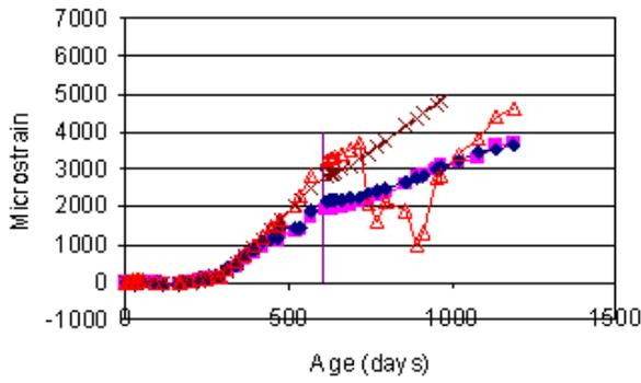
Pile 10- Steam curing, half-immersed in water. Hr aggregate, 2.6% SO<sub>3</sub>
