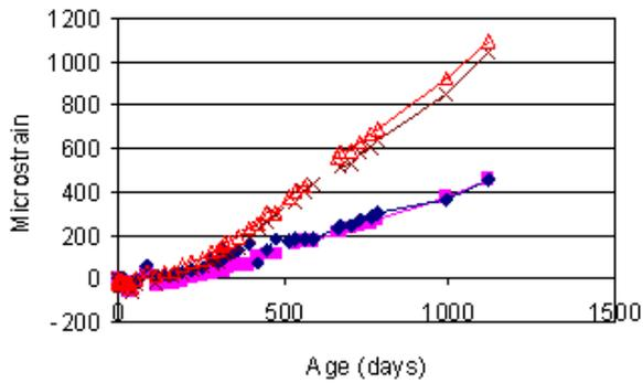
Normal curing, half-immersed in salt solution, Lr aggregate
