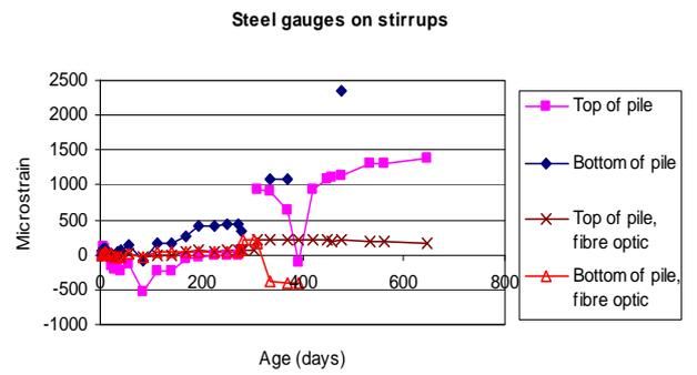
Figure 16: Comparison of readings from the fibre optic and electrical foil gauges installed on steel bars in Pile 12.
