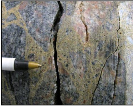
Figure 2: Concrete core, Pointe du Bois GS, showing ASR gel deposits associated with granite aggregate
