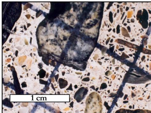
Figure 6: Damage Rating Index sample of polished concrete, showing ASR-gel-filled crack and reaction rims on aggregate.
