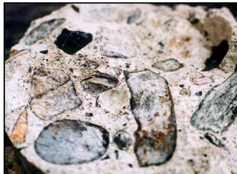
Figure 7: ASR gel, reaction rims on aggregates on sample of concrete from dam, Southern BC.
